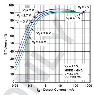
Figure 4. Efficiency vs Output Current, TPS62240
