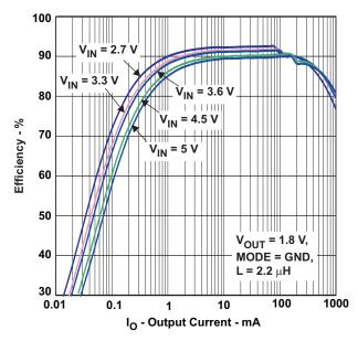
Figure 3. Efficiency vs Output Current, TPS62290
