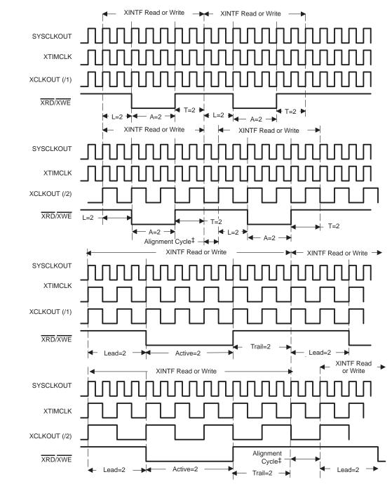
Figure 10. XTIMCLK and XCLKOUT Mode Waveforms
