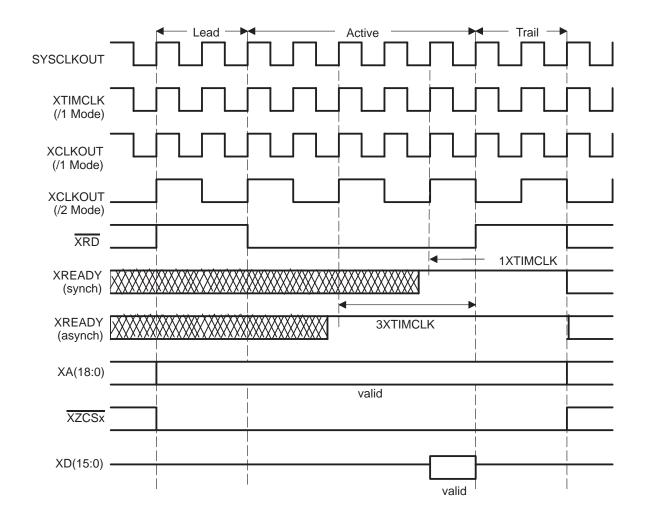
Figure 11. Generic Read Cycle (XTIMCLK = SYSCLKOUT mode)<sup>†</sup>
