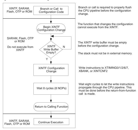
Figure 4. Access Flow Diagram
