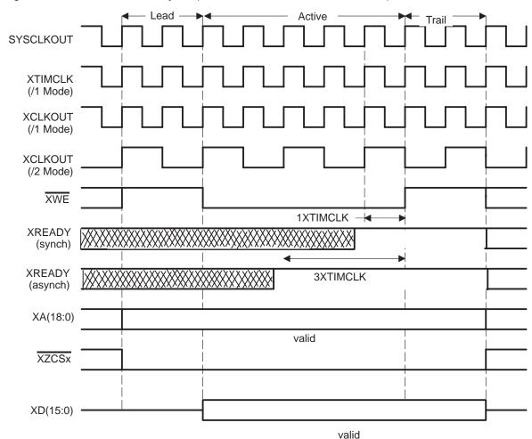
Figure 13. Generic Write Cycle (XTIMCLK = SYSCLKOUT mode)<sup>†‡</sup>
