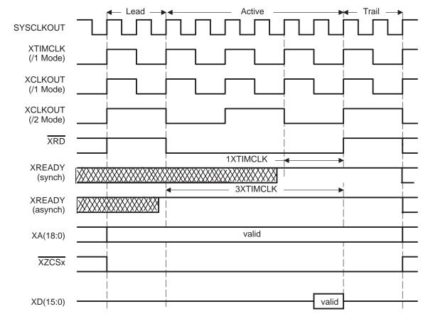
Figure 12. Generic Read Cycle (XTIMCLK = 1/2 SYSCLKOUT mode)<sup>†</sup>
