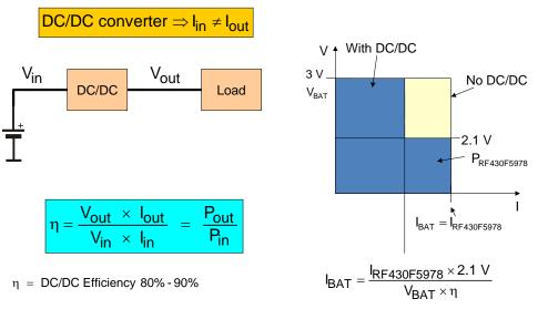
Figure 15. DC/DC Converter Scheme
