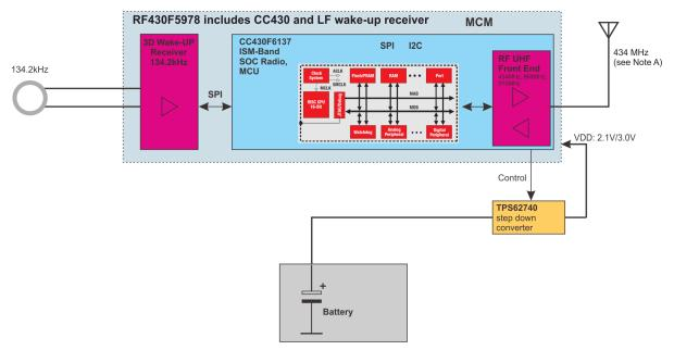
A 434-MHz worldwide frequency depends on the RF430F5978EVM RF filter and the selected UHF frequency condition. With different hardware, the kit can use the 315-, 868-, or 915-MHz bands.
