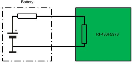
Figure 12. RF430F5978 Battery Supply
