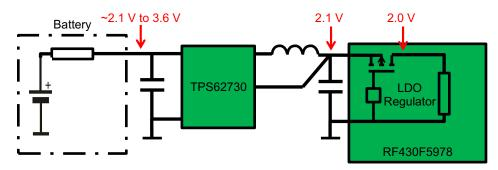
Figure 16. RF430F5978 TPS62730 Supply With Voltage Levels
