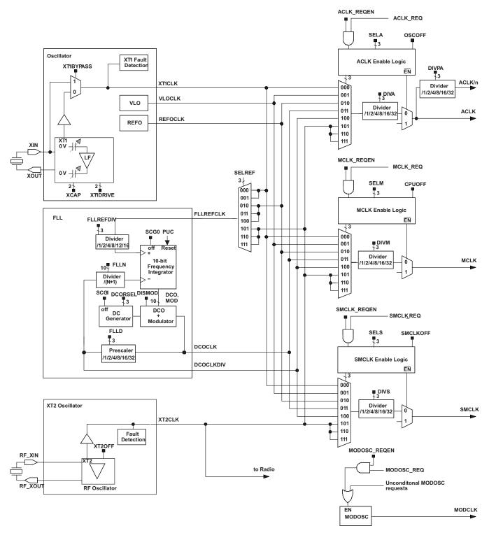
Figure 11. RF430F5978 Unified Clock System
