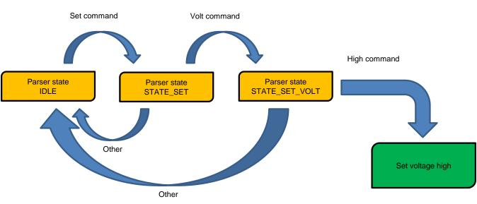
Figure 9. Parser Example Flowchart
