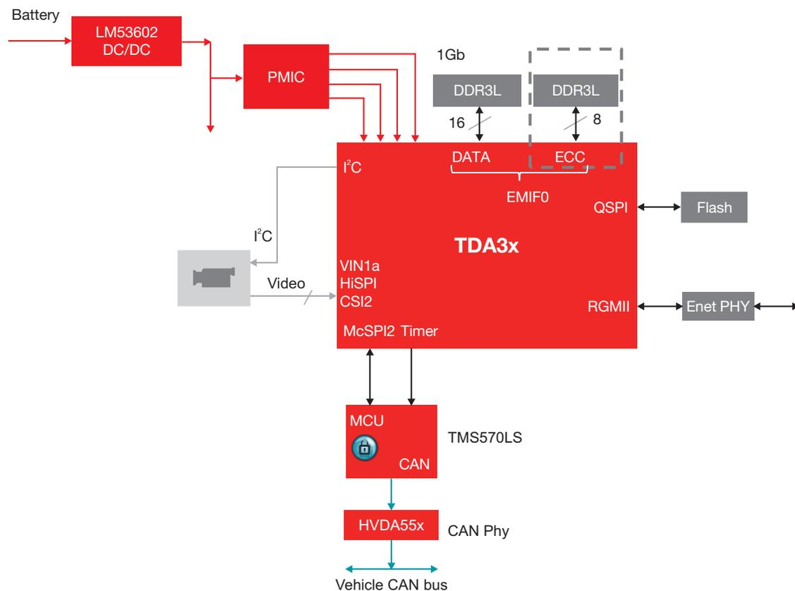
**Figure 1.** Front camera block diagram with TDA3x SoC processor.
