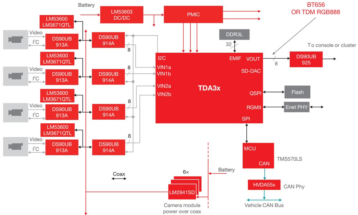
Figure 2. Surround view solution on TDA3x SoC processor.
