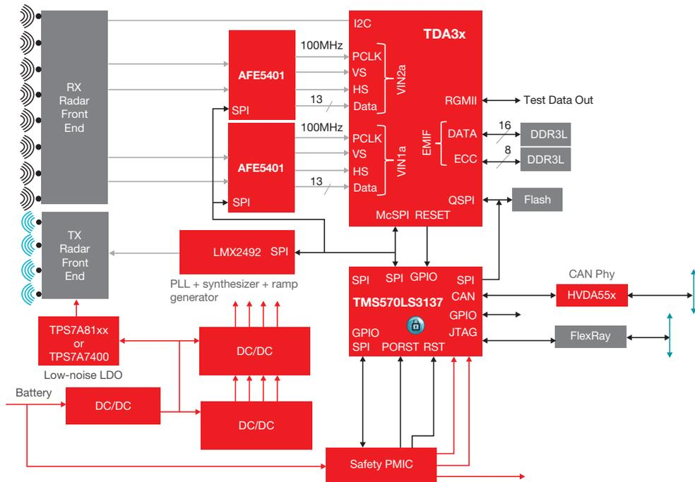
**Figure 4.** Radar on a TDA3x processor.
