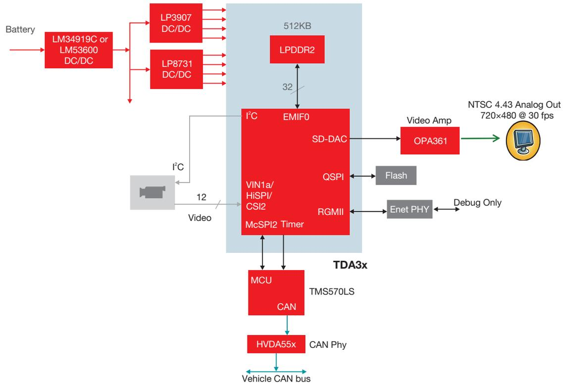
**Figure 3.** Size-constrained ADAS camera on a TDA3x processor.
