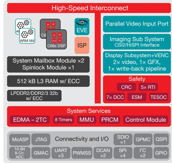
Figure 5. TDA3x processor block diagram.
