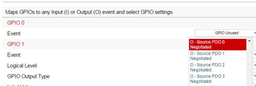
**Figure 2. Discrete GPIO Events Named “Source PDO # Negotiated”**
