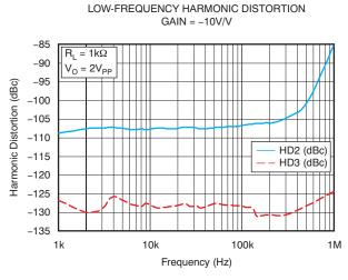
Figure 9. OPA847 Low-Frequency Harmonic Distortion (Gain of –10V/V)
