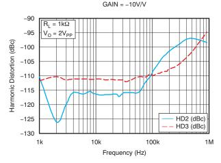
Figure 10. OPA683 Low-Frequency Harmonic Distortion (Gain of -10V/V)
