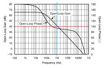
Figure 1. OPA890 Open-Loop Gain and Phase Performance
