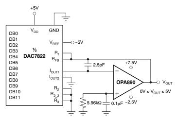
Figure 15. Multiplying DAC Transimpedance Driver
