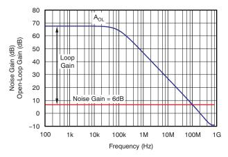
Figure 3. VFA Loop Gain (Typical Performance)
