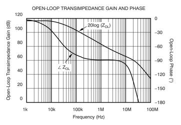
Figure 7. OPA683 Open-Loop Transimpedance Gain Performance
