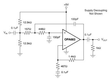
Figure 13. Single-Supply Sallen-Key Filter Implementation
