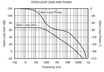
Figure 8. OPA2889 Open-Loop Gain Performance
