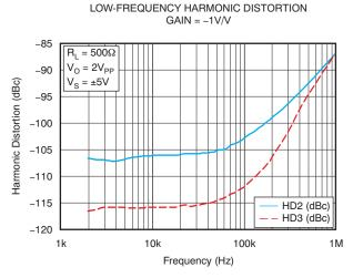
Figure 5. OPA2889 Low-Frequency Harmonic Distortion (Gain of -1V/V)
