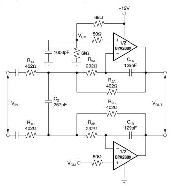
Figure 11. MFB Filter Topology Using the OPA2889
