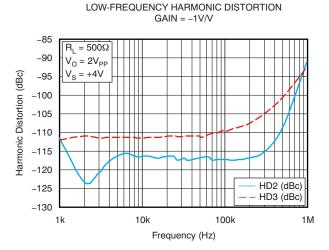
Figure 6. OPA683 Low-Frequency Harmonic Distortion (Gain of -1V/V)
