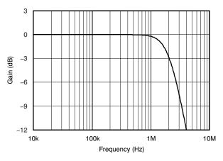
Figure 12. MFB Filter Frequency Response
