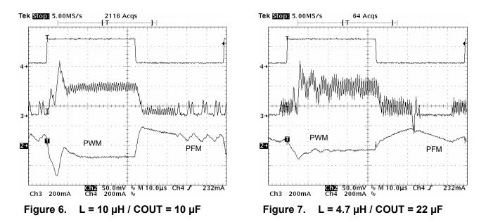
TPS62204 load transient performance vs L-C filter combination 3.6-V input voltage / 1.6-V fixed output voltage
