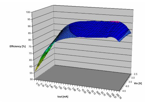
Figure 5. TPS62204 (1.6V) Efficiency vs Load Current vs Input Voltage With 4.7- $\mu$ H Wire-Wound Inductor, R<sub>dc</sub> = 240 m $\Omega$  / I<sub>SAT</sub> = 700 mA
