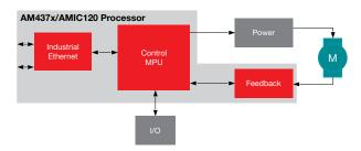
*Figure 6:* Single-chip robot controller system based on AM437x or AMIC120 processors.
