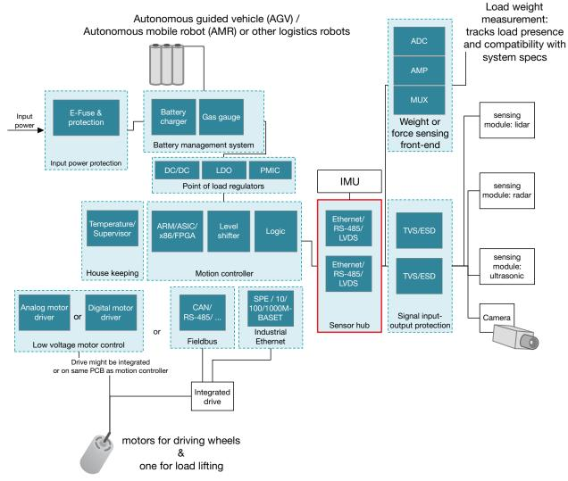
Figure 2: High level block diagram for an autonomous guided vehicle or robot.
