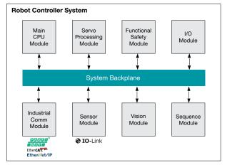
Figure 4: Robot controller system example for high-end industrial robots.
