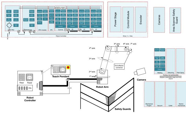
Figure 1: Typical system components in an industrial robot system.
