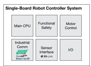
*Figure 5:* Single-board robot controller system for collaborative or SCARA robots.
