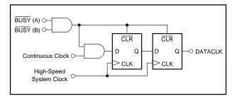
FIGURE 5. Gating a Continuous Clock with a Worst-Case BUSY. (Recommended method.)
