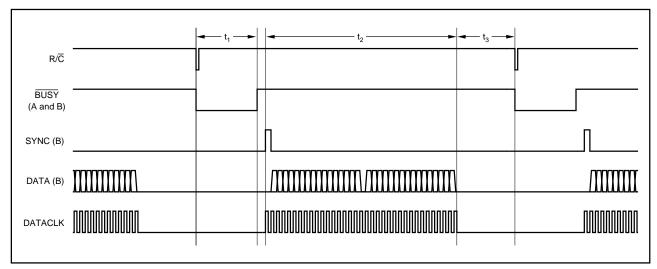
FIGURE 6. Multiple Conversions for the Converters Shown in Figure 1.
