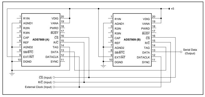
FIGURE 1. Two ADS7809s Utilizing the Tag Feature.
