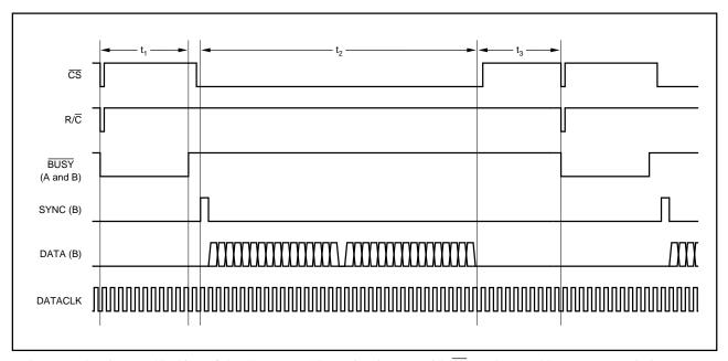
FIGURE 7. Continuous Clocking of the Converters Shown in Figure 1 with  $\overline{CS}$  used to Enable Data Transmission.
