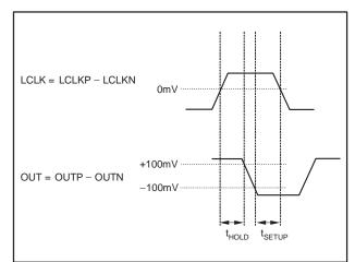
Figure 2. Setup and Hold Times
