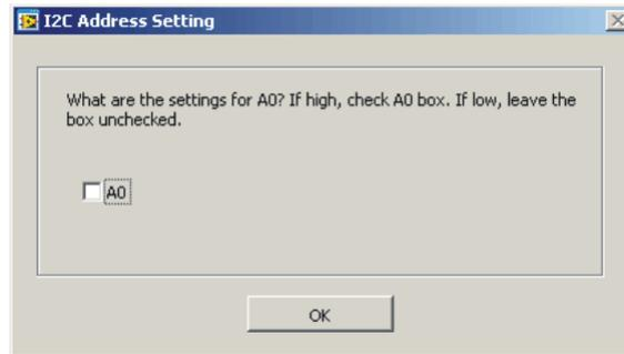
**Figure 2. Prompt to Set Up TSC2014 I<sup>2</sup>C Slave Address**
