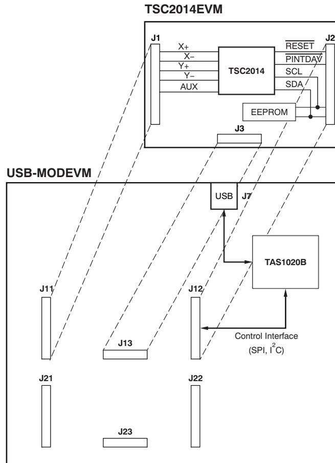
Figure 1. TSC2014EVM-PDK Hardware Block Diagram and Connection
