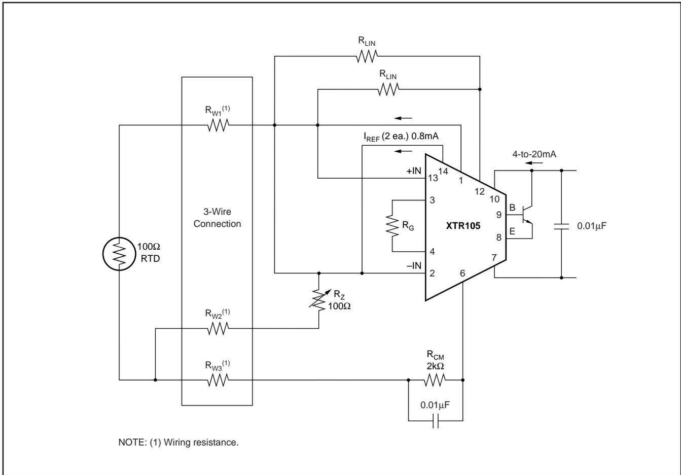
FIGURE 2. Three-Wire RTD to 4-to-20mA, Two-Wire Transmitter using XTR105. When the RTD is located remotely, this “three-wire” solution can improve accuracy. For linearization, a second resistor is required with this solution. See the XTR105 data sheet for additional details.
