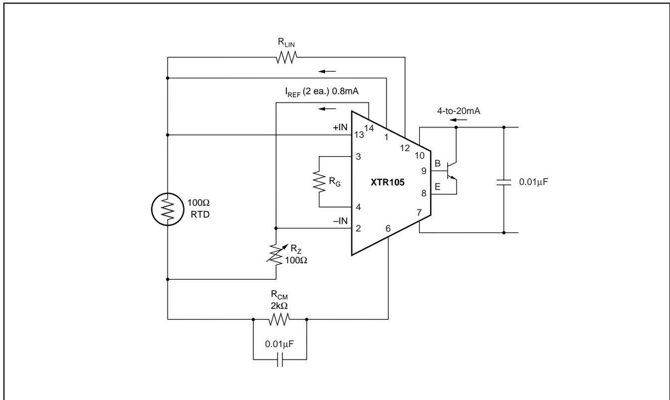
FIGURE 1. Basic RTD to 4-to-20mA Two-Wire Transmitter Using XTR105. Internal 0.8mA current sources excite the RTD and zero-setting resistor.  $R_{CM}$  provides additional voltage drop to set the XTR105 inputs within their valid common-mode input range. Optional resistor,  $R_{LIN}$  can be used for linearization of the RTD. See the XTR105 data sheet for additional details.
