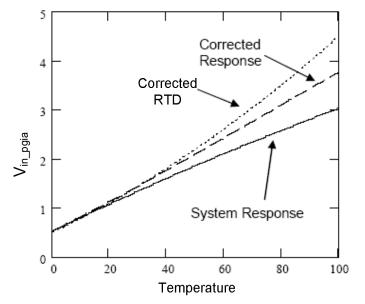
$$V_{in_pgia} = \left(K_{lin} V_{in_pgia} + I_{ref}\right) \left(RTD - R_{z}\right)$$
