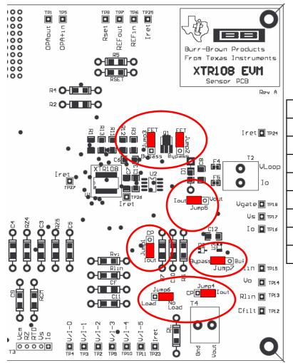
The table below and the figure illustrate the jumper settings for current output mode calibration.
