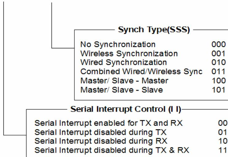
**Figure 15. Synchronization Type and Interrupts**
