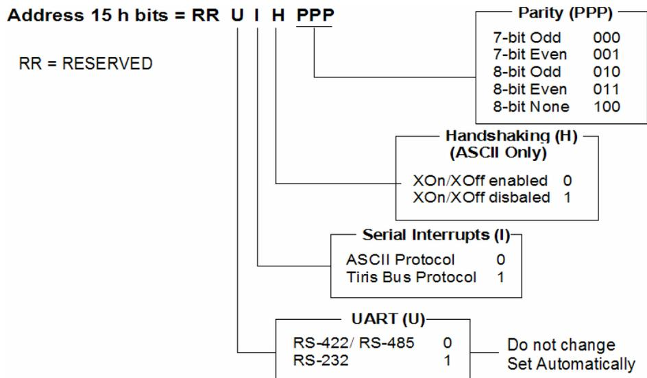
**Figure 13. Communications Parameters**
