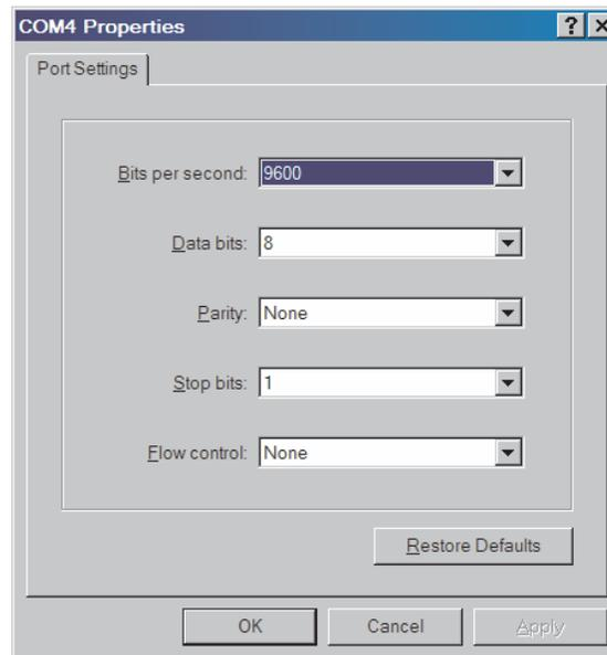
**Figure 7. COM Port Parameters**
