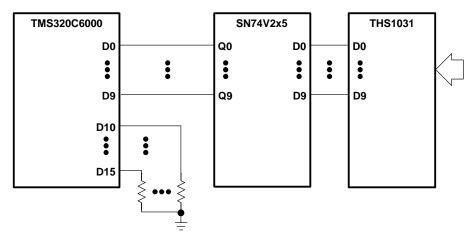
Figure 13. Pulldown Resistor for Unused Input Data Pins
