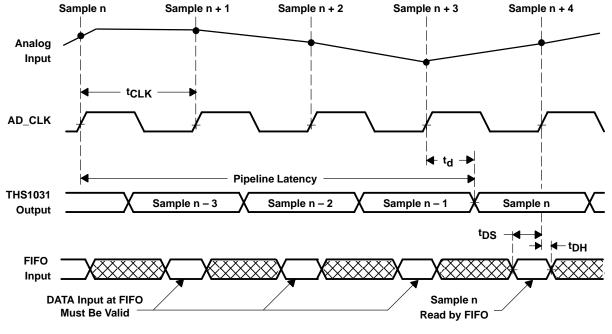
Figure 9 shows the timing between the ADC and the FIFO.
