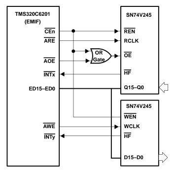
Figure 4. SN74V2x5-to-EMIF Interface With Glue Logic
