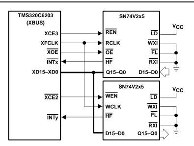
Figure 7. Glueless SN74V2x5-to-XBUS Interface
