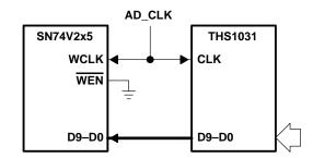
Figure 8. Simple ADC-to-FIFO Interface
