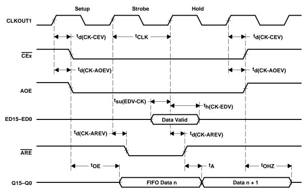
Figure 5. 'C6201 DSP Asynchronous Read Timing (Single Read)
