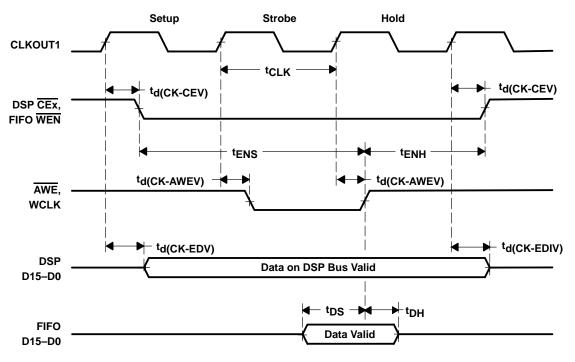
Figure 6. 'C6201 DSP Asynchronous Write Timing (Single Write)
