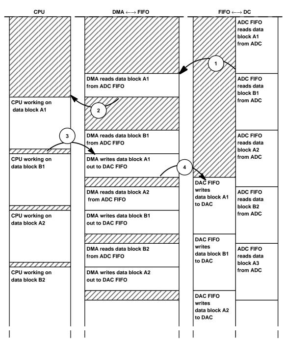
Figure 12. Software Flow in a Simple Application
