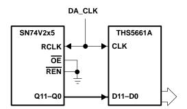
Figure 10. Simple DAC-to-FIFO Interface
