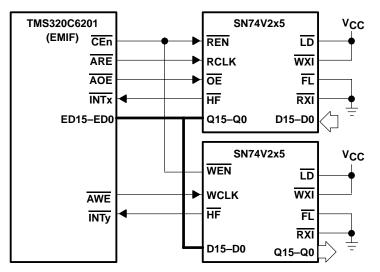
NOTE A: This configuration can be used only if no other devices are using the asynchronous control signals or if the FIFO is used only as an output buffer, not for input. The DSP must offer separate control lines for the asynchronous and synchronous memory types (C6x0x).
