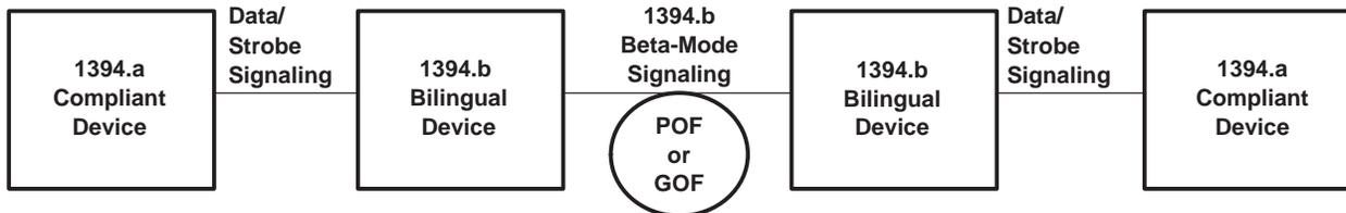
**Figure 1. IEEE-1394 Mixed (1394.a and 1394.b) Network**
