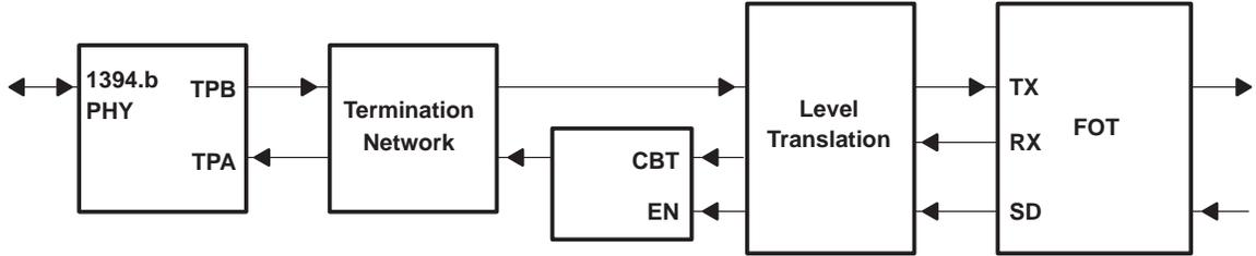
Figure 4. Basic Fiber-Optic Components
