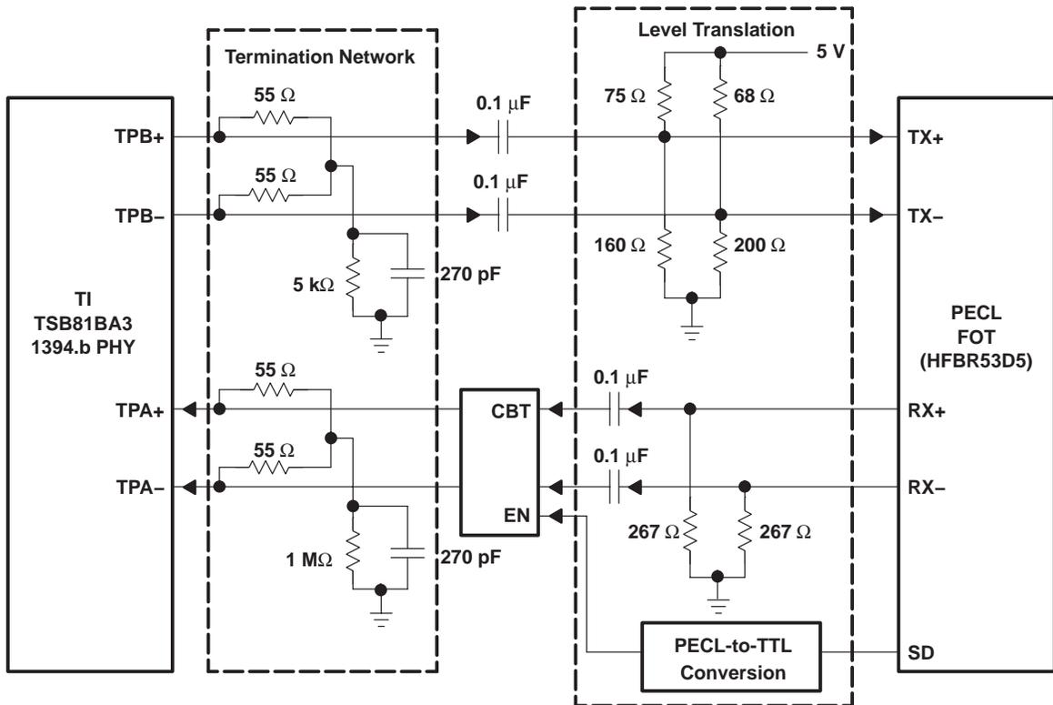
Figure 5. Connections to PECL FOT
