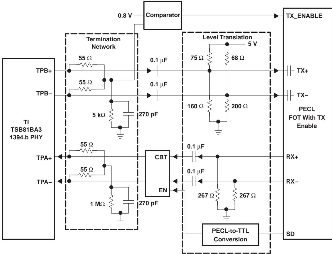
Figure 7. Connections for Internally AC-Coupled PECL FOT With Transmit Enable
