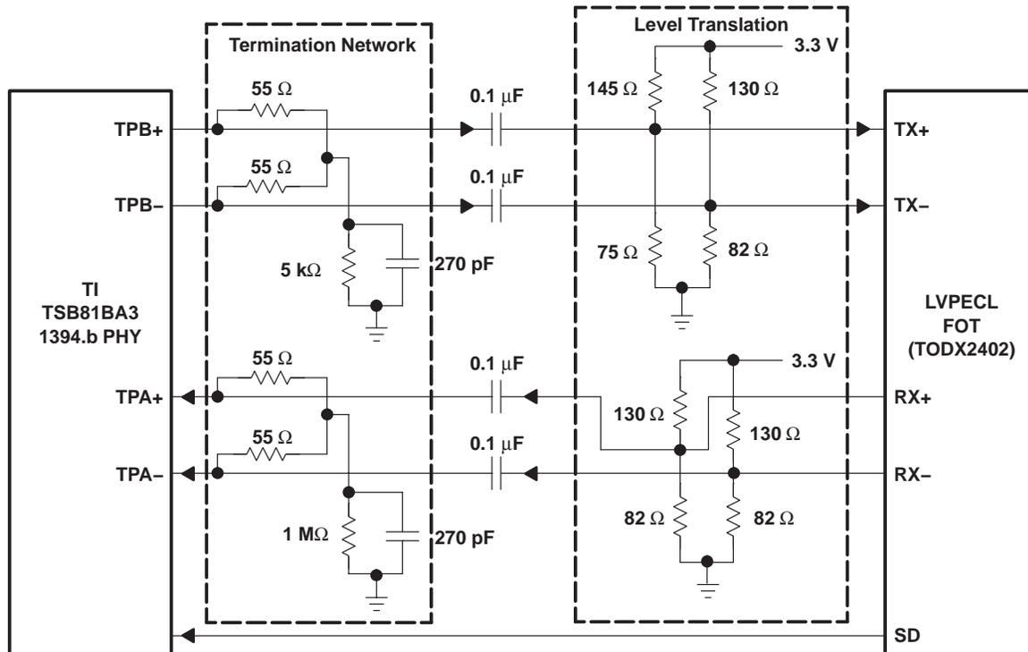
Figure 6. Connections to LVPECL FOT
