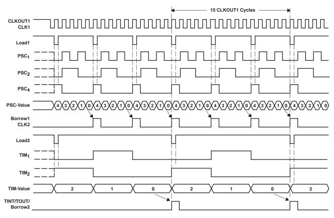
Figure 18. Timing Diagram for TDDR = 4 and PRD = 2
