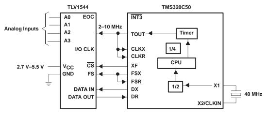
Figure 11. Glueless Interface for Low-Volt Operation
