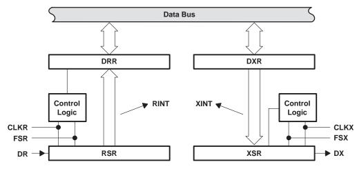
Figure 12. Serial Port Block Diagram
