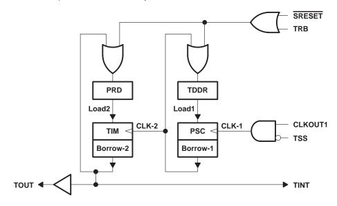
Figure 17. Timer Block Diagram
