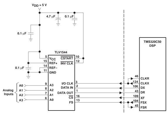
NOTE: Fixed data clock is only possible with  $V_{DD} = 5 V$ .
