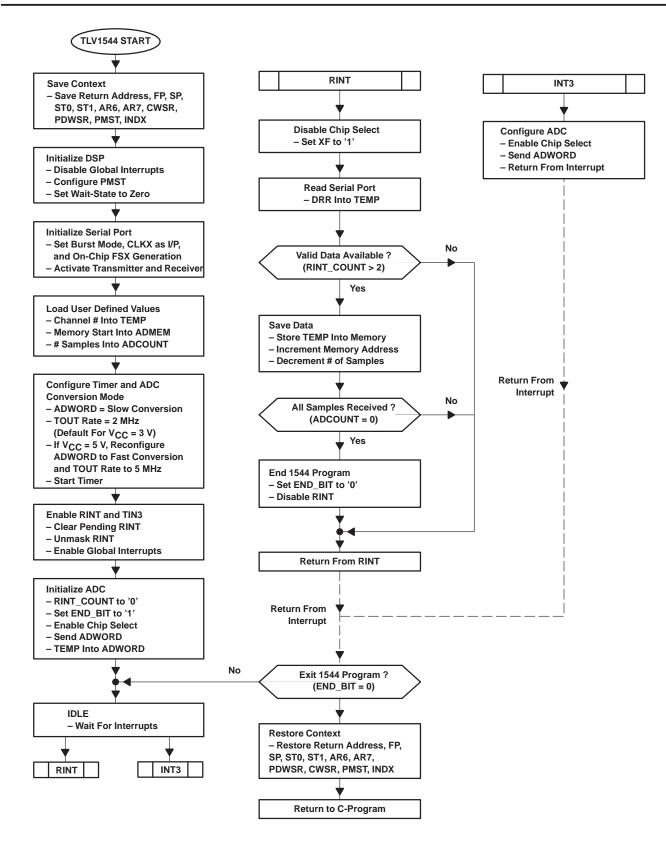
Figure 25. Flowchart of C1544CLK.asm (Timer as Clock Source)
