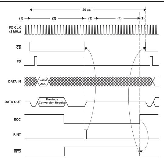
Figure 24. Data Transfer Sequence When Using INT3 and ADC in Slow Conversion
