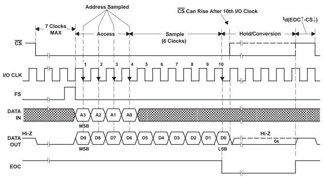
NOTES: E. The falling edge of FS has to appear within 7 I/O clock cycles from the falling edge of  $\overline{CS}$ .
