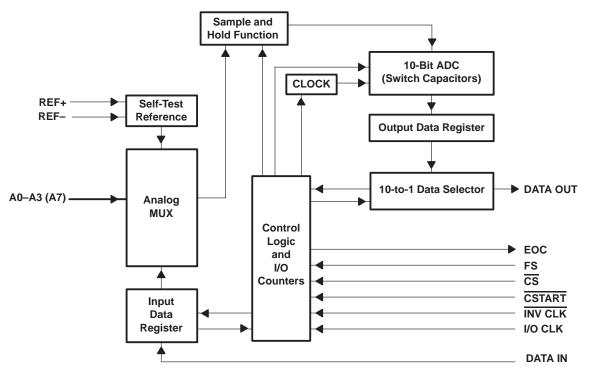
Figure 6. Functional Block Diagram of the TLV1544 and TLV1548
