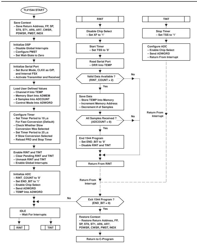
Figure 22. Flowchart of C1544IN.asm (Timer as Interrupt Source)
