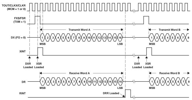
Figure 16. Transmit and Receive Operation in Burst Mode
