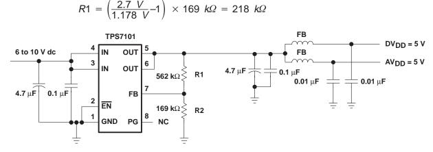
NOTES: A. R1 = 562 k $\Omega$  for V\_DD = 5.1 V and 218 k $\Omega$  for V\_DD = 2.7 V
