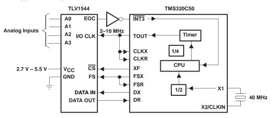
Figure 23. External Interrupt, INT3, Detects EOC Via External Inverter
