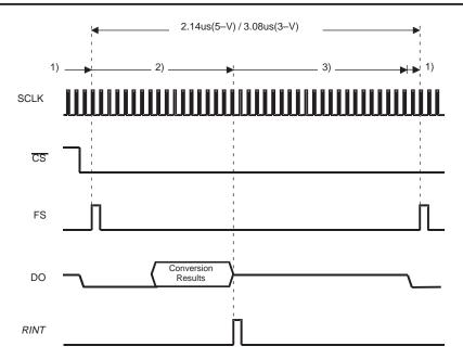
Figure 9. Interface Timing Using RINT
