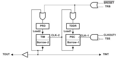
Figure 7. Timer Block Diagram
