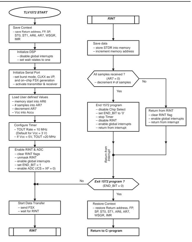
Figure 10. Flowchart of TLV1572.asm
