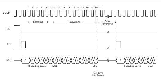
Figure 4. ADC/DSP Interface Timing
