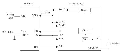
Figure 8. ADC/DSP Interface
