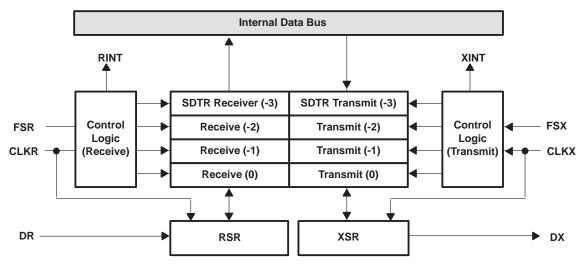
Figure 5. Synchronous Serial Port Block Diagram
