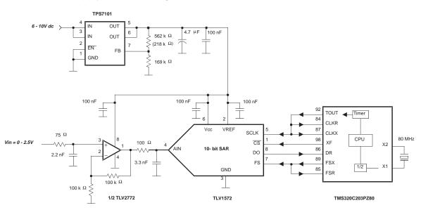
Figure 2. Mini Data Acquisition System
