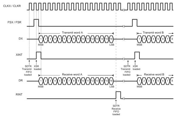
Figure 6. Transmit- and Receive-Operation in Burst Mode
