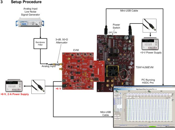
Figure 2. EVM Test Setup
