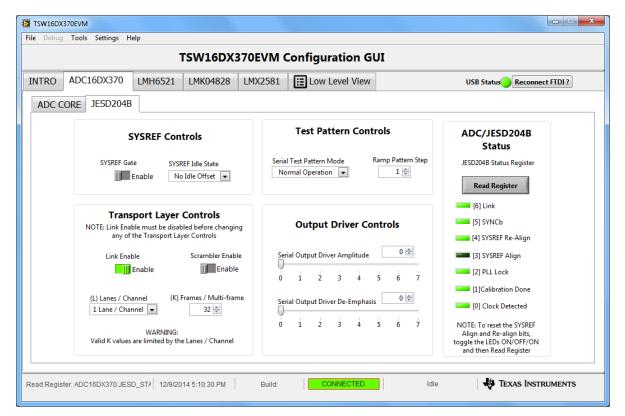
Figure 6. Configuration GUI JESD240B Tab
