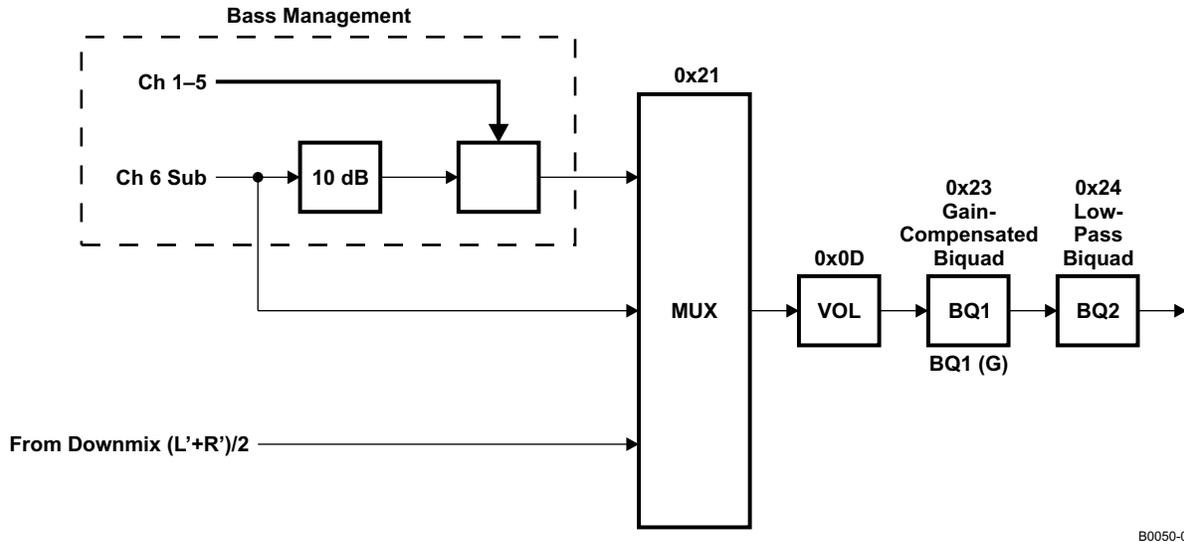
Figure 4. Channel-6 (Subwoofer) Processing Block Diagram
