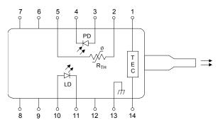
Figure 2: Pump Laser Module
