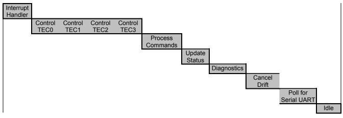
Figure 5: Task Flow Diagram
