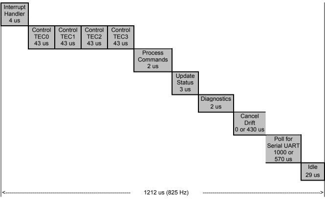
Figure 16: Overall Timing Diagram
