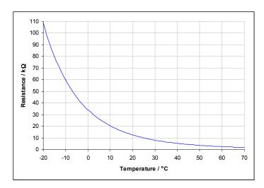
Figure 3: Example Thermistor Resistance as a Function of Temperature
