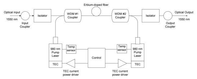
Figure 1: Dual-Pumped EDFA Basic Block Diagram
