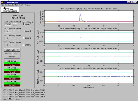
Figure 11: Response to -8°C Setpoint Temperature Step
