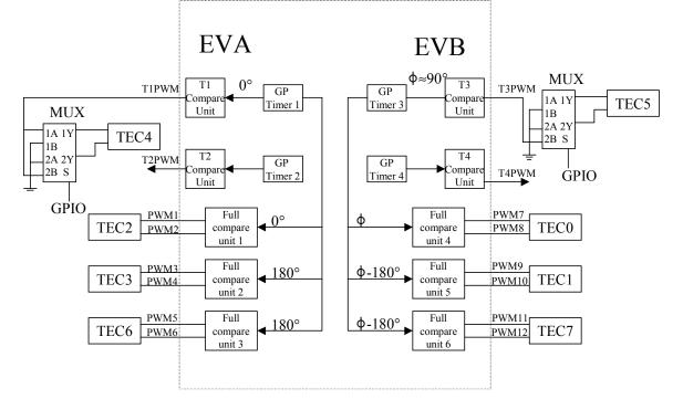
Figure 17: PWM DAC Configuration for Eight TEC Channels
