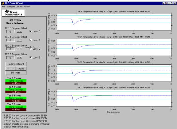
Figure 14: Response to Changing Ambient Temperature from Hot to Cold
