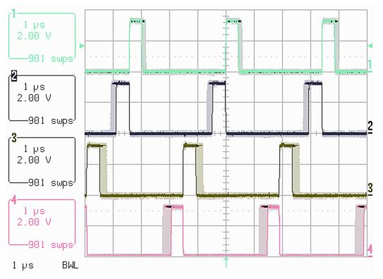
Figure 8: PWM Phase Alignment
