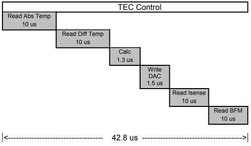
Figure 6: Detailed TEC Control Timing
