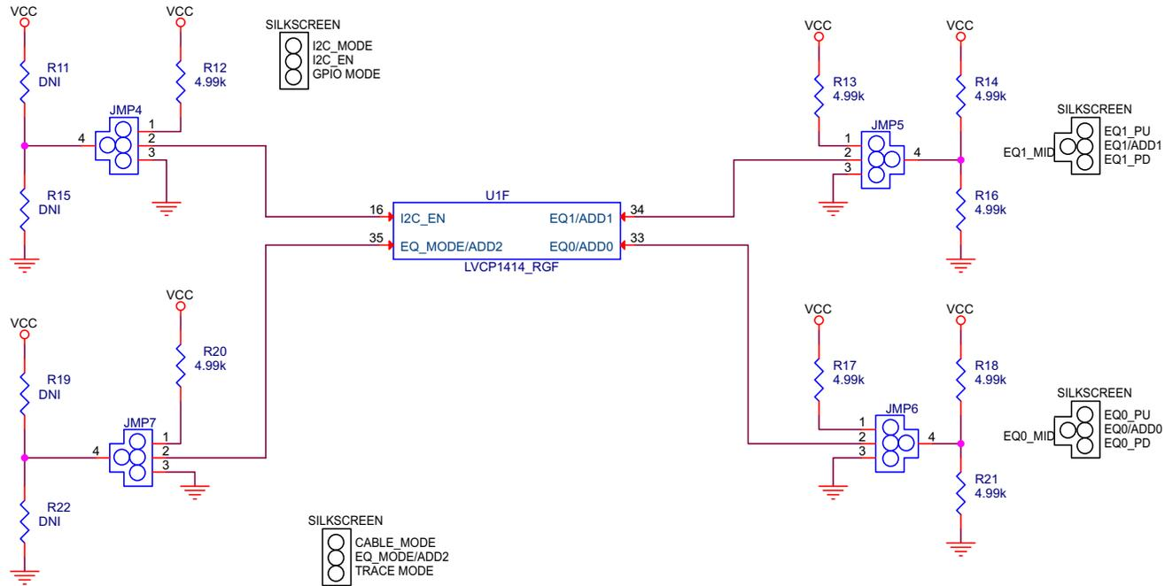
Figure 6. SN65LVCP1414 EVM Schematic, Sheet 3 I<sup>2</sup>C Controls
