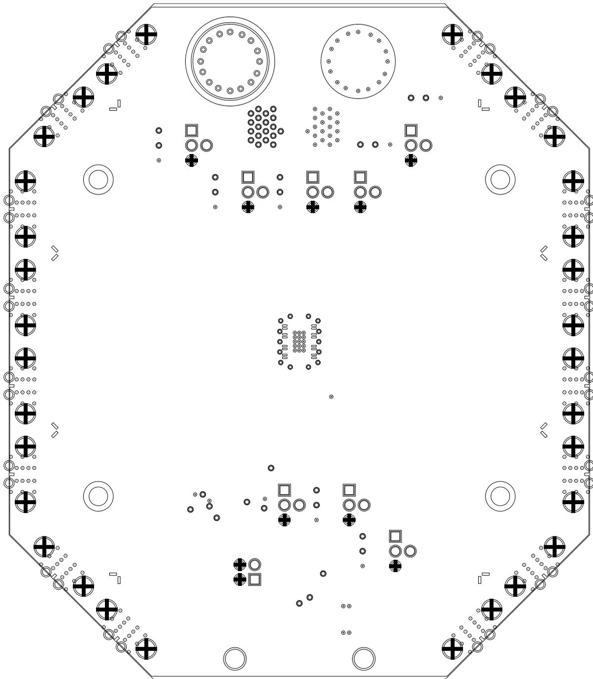
**Figure 10. SN65LVCP1414 Board Layout: Internal Ground (Layer 2)**
