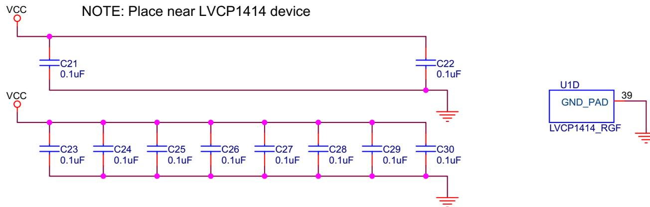
Figure 8. SN65LVCP1414 EVM Schematic, Sheet 5 Power
