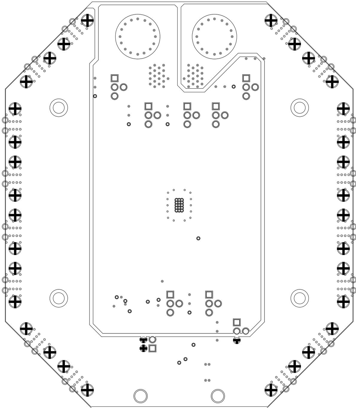
**Figure 11. SN65LVDS1414 EVM Board Layout: Internal Power (Layer 3)**
