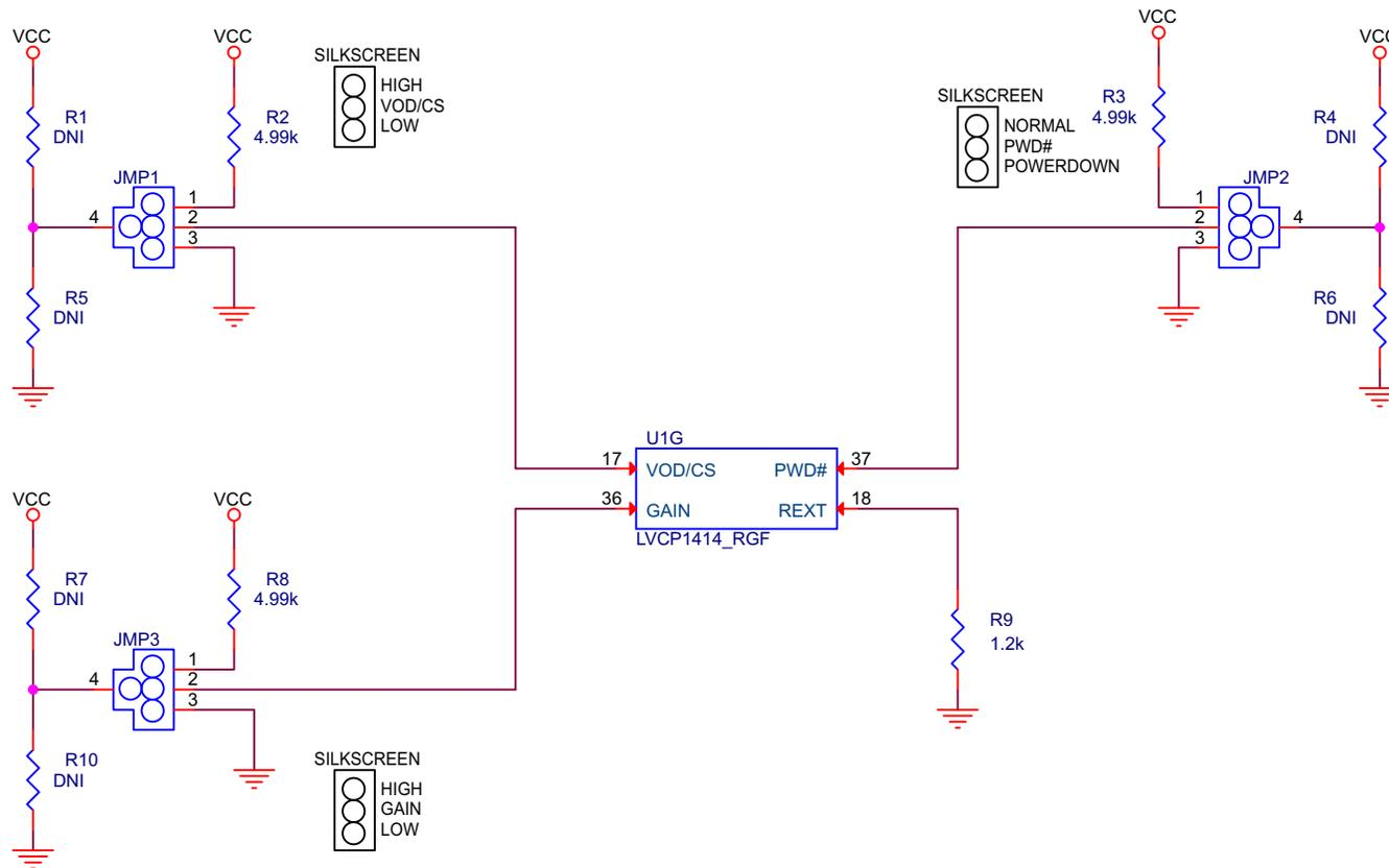
Figure 5. SN65LVCP1414 EVM Schematic, Sheet 2 GPIO Controls
