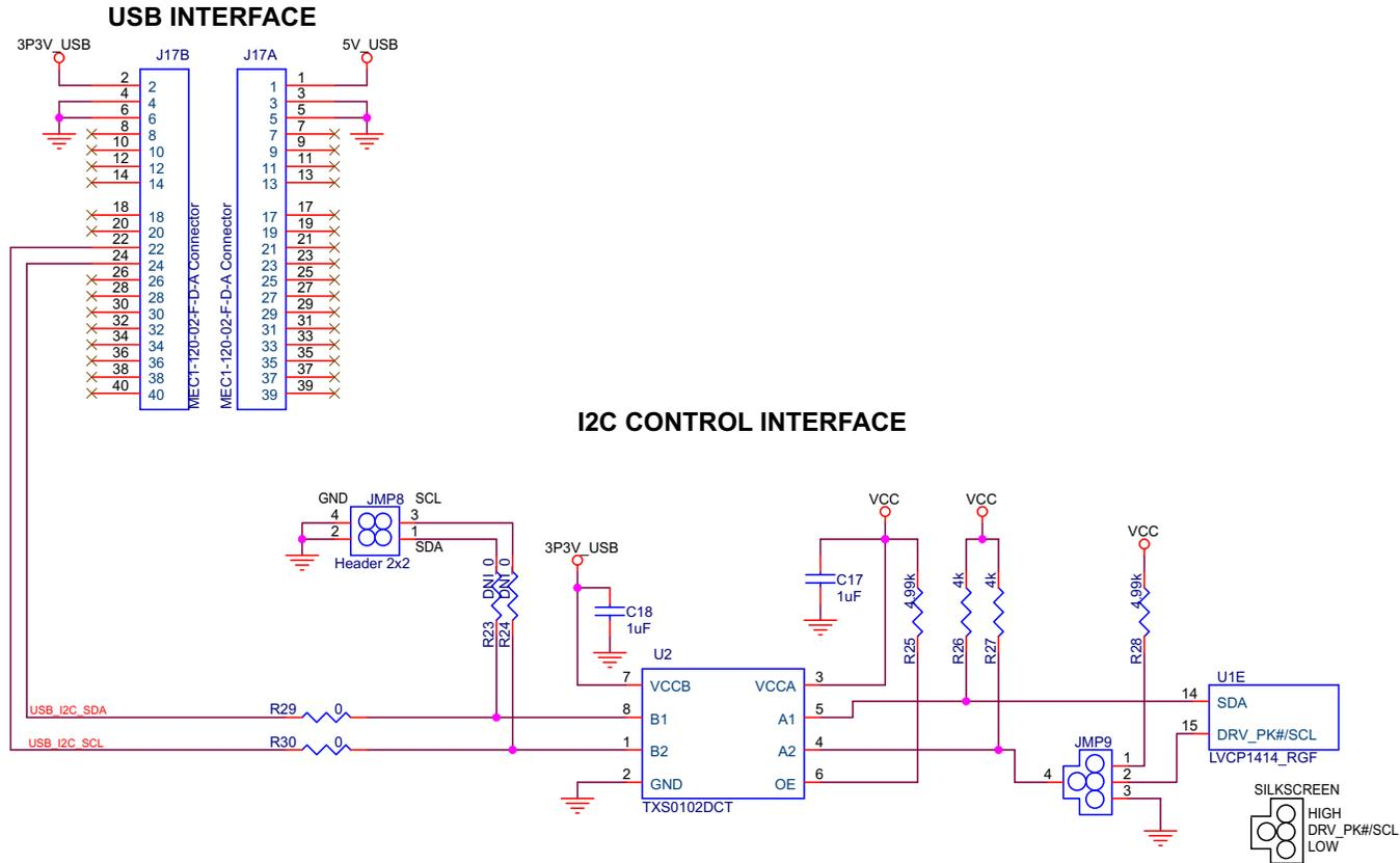
Figure 7. SN65LVCP1414 EVM Schematic, Sheet 4 I<sup>2</sup>C Communications
