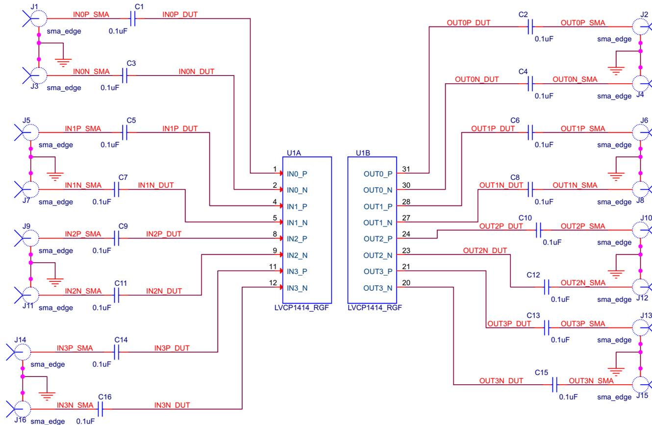
Figure 4. SN65LVCP1414 EVM Schematic, Sheet 1 Inputs and Outputs
