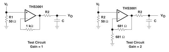
Figure 1. Test Circuits
