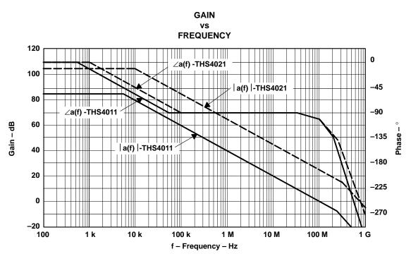
Figure 1. Open-Loop Gain and Phase – THS4011 and THS4021
