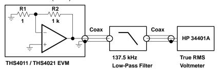
Figure 15. Noise Test Setup
