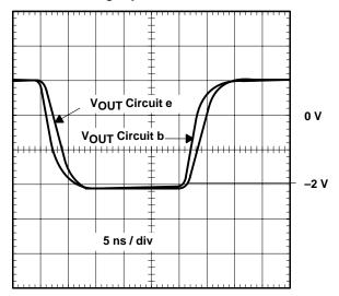
Figure 14. Transient Response – Inverting Amplifiers
