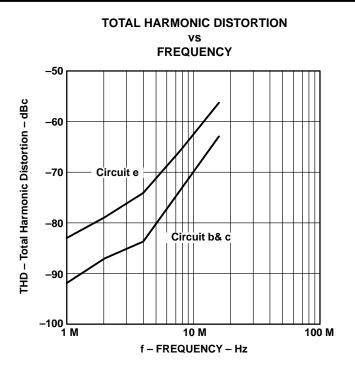
Figure 12. THD vs Frequency – Inverting Amplifiers, V<sub>OUT</sub> = 2 Vp-p
