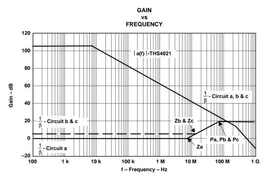
Figure 8. Plot of Open-Loop and Inverse-Feedback Factors of Test Circuits
