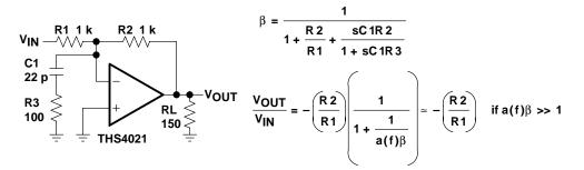
Figure 5. Circuit c: One-Capacitor, Externally-Compensated, THS4021 – Inverting Amplifier
