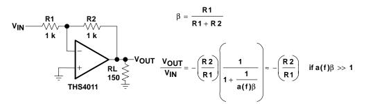
Figure 7. Circuit e: Internally-Compensated THS4011 – Inverting Amplifier
