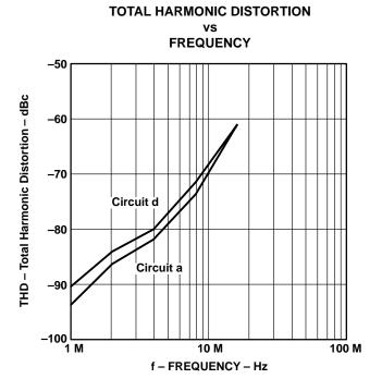
Figure 11. THD vs Frequency – Noninverting Amplifiers, V<sub>OUT</sub> = 2 Vp-p
