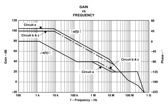
Figure 9. Plot of Magnitude and Phase of  $|a(f)|\beta$  – Circuits a, b, and c
