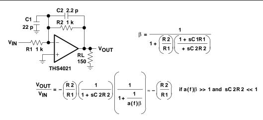
Figure 4. Circuit b: Two-Capacitor, Externally-Compensated, THS4021 – Inverting Amplifier
