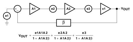
Figure 2. Model of Operational Amplifier With Negative Feedback
