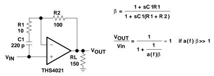
Figure 3. Circuit a: Externally-Compensated THS4021 – Noninverting Amplifier
