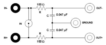
Figure 2. Schematic of the RC Low-Pass Filter for One Channel
