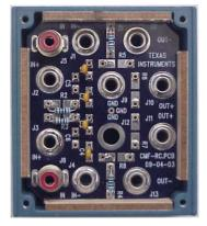
Figure 3. Top and Inside View of Texas Instruments RC Filter Box
