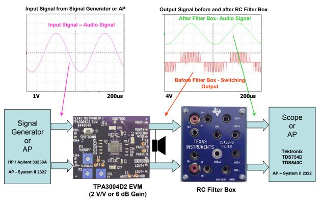
Figure 1. Filter Box Setup for Output Power Measurement
