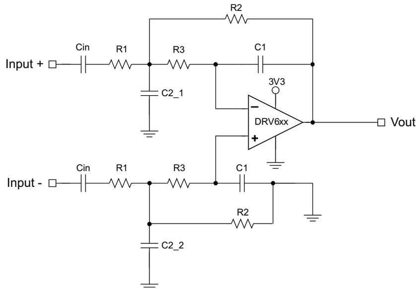
Figure 2. Circuit for Interfacing to Differential Output DAC
