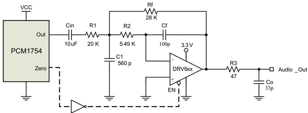
**Figure 4. Interfacing DRV6xx to PCM1754**
