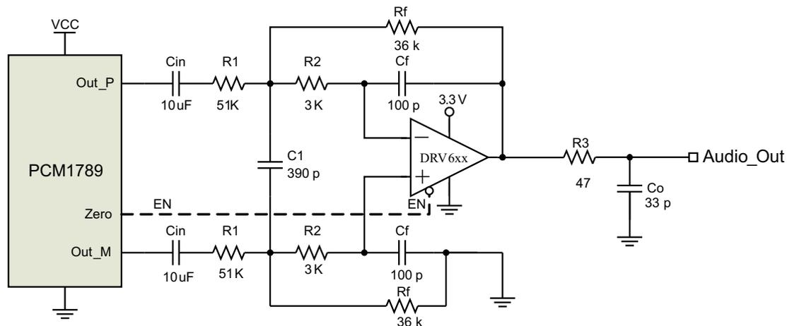
Figure 5. Interfacing DRV6xx to PCM1789
