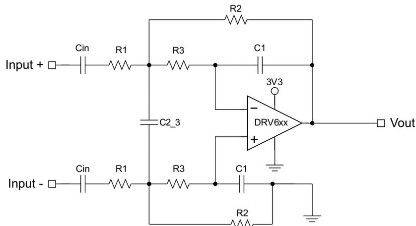
**Figure 3. Simplified Circuit for Interface to Differential Output DAC**
