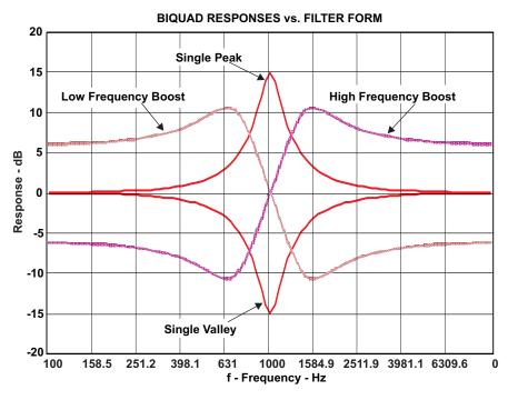
Traces in the graph that follows illustrate something of the range of responses a biquad filter can generate. The responses are arranged as follows for clarity.
