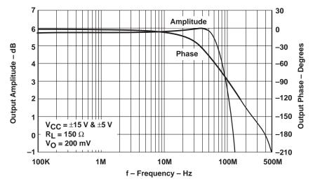
Figure 1–4 shows the typical frequency response of the THS4011 EVM using the inverting input (G = –1). Typical –0.1 dB bandwidths are 30 MHz and a –3-dB bandwidth of 83 MHz with a  $\pm$  15 V power supply. These bandwidths remain consistent when the power supply drops to  $\pm$ 5 V.
