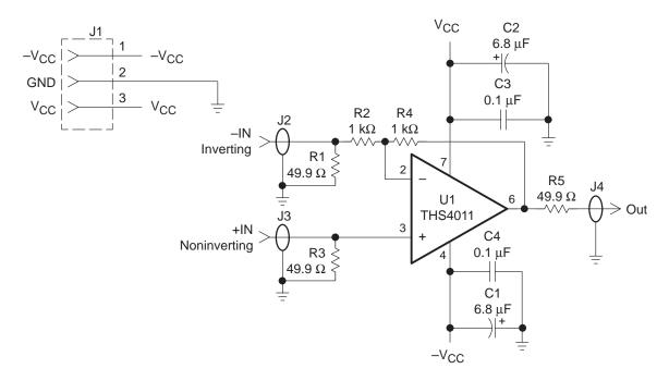
The gain of the EVM inputs can easily be changed to support a particular application by simply changing the ratio of resistors R1, R4, and R5 as described in the following equations:
