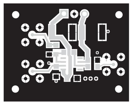
Figure 2–2. THS4011 EVM PC Board Layout – Component Side
