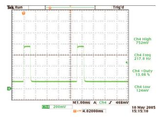
Figure 2. GSM Load Profile Across a 0.5- $\Omega$  Resistor
