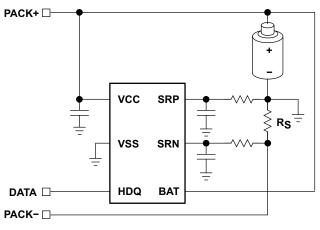
Figure 1. Simplified Gas Gauge Circuit
