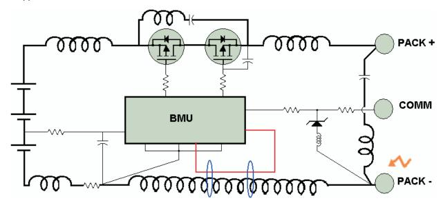
Figure 9. Avoid Close Spacing Between High Current and Low Level Signal Lines
