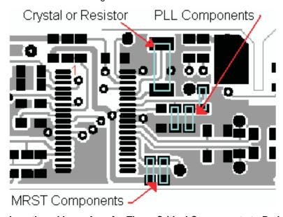
Figure 2. Minimize Length and Loop Area for These Critical Components to Reduce Noise Pickup.
