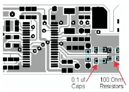
Figure 7. Differential Filter Components With Symmetrical Layout.
