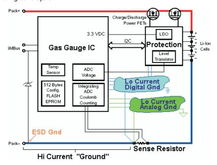
Figure 4. Use Separate Analog and Digital Low-Current Ground Systems
