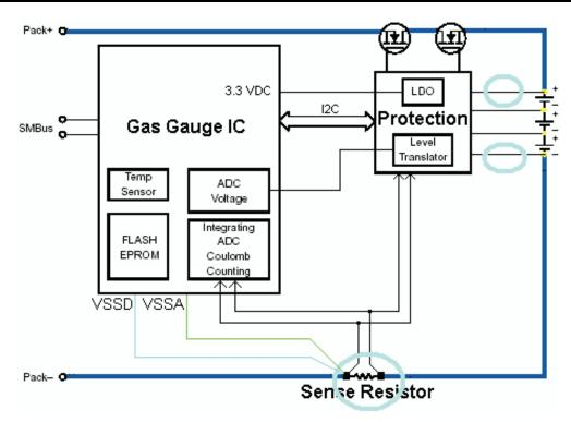
Figure 6. Fig 6. RIGHT! In Some Cases, Top and Bottom Cell Voltage Sensing may be Extended out to the Cells.
