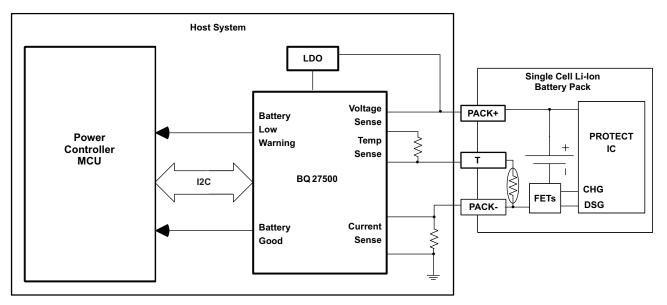
Figure 1. bq27500 Host-Side Battery Fuel Gauge
