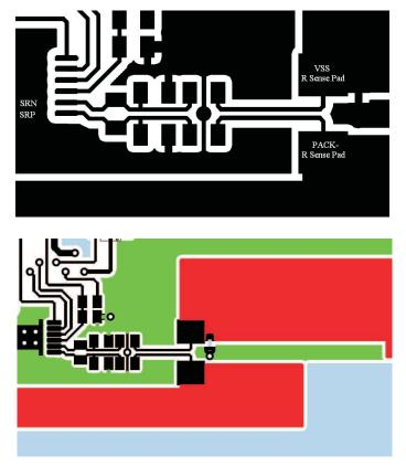
Figure 6. Sense-Resistor Connection and Grounding
