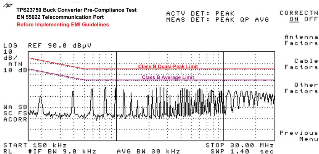
**Figure 1-8. Conducted Emissions Before Implementing EMI Guidelines**
