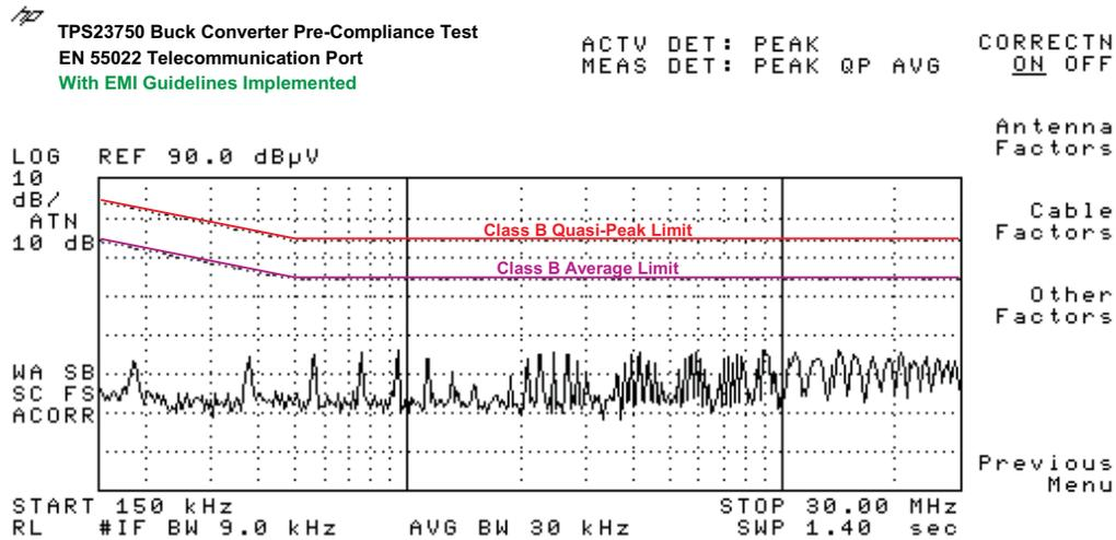
**Figure 1-7. TPS23750 Buck Converter Conducted Emissions Results**
