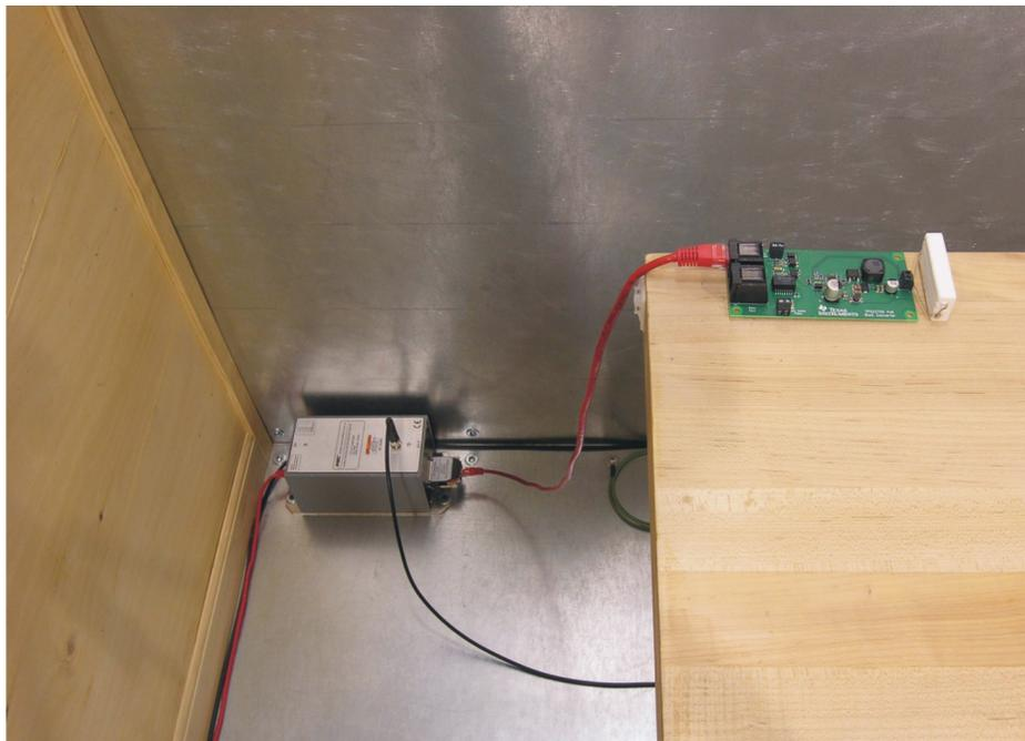
Figure 1-6. Conducted Emissions Pre-Compliance Test Setup Photo
