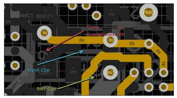
Figure 8. bq25120 Capacitors Placement
