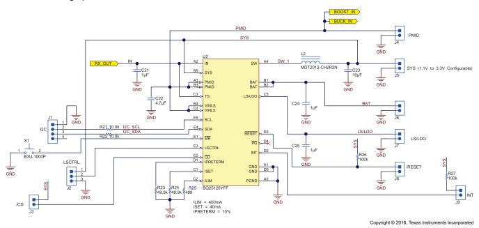
Figure 4. Schematic of Battery Charger, MCU, Radio, and Sensor Power
