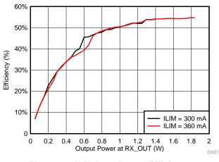
Figure 14. Wireless Power Efficiency
