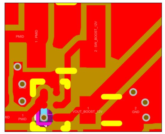
Figure 10. Capacitor Grounding TPS61046
