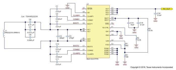
Figure 3. Schematic of Wireless Charging Receiver Using the bq51003
