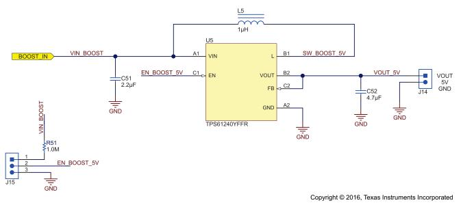
Figure 7. Schematic of Boost for Heart Rate Monitor Power
