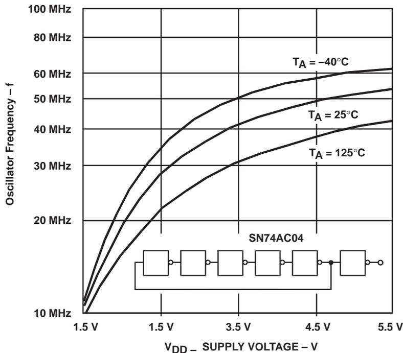
Figure 9. Output Frequency of the Ring Oscillator
