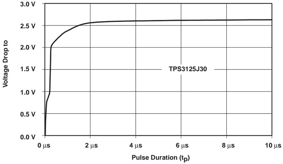
Figure 12. TPS3125J30—Reaction fo Voltage Drops
