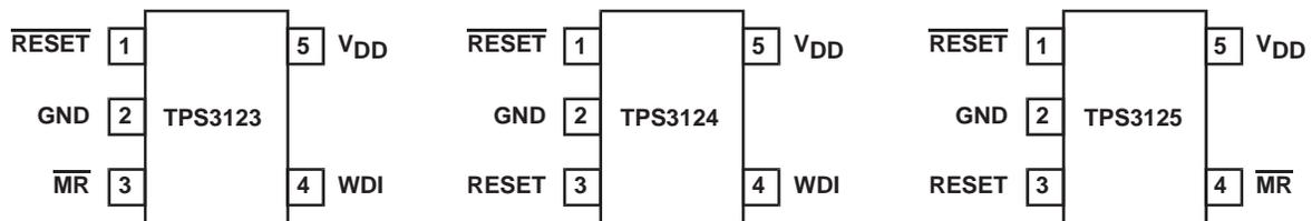
**Figure 4. Terminal Assignments of TPS312x Series Circuits**
