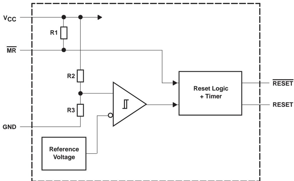
Figure 5. TPS3125 Supply Voltage Supervisor
