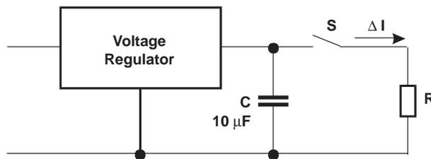
**Figure 10. Load Change in the Power Supply**
