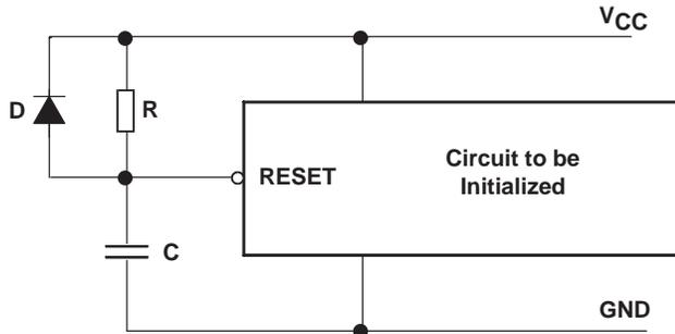
**Figure 1. Circuit for Generating Reset Signals**
