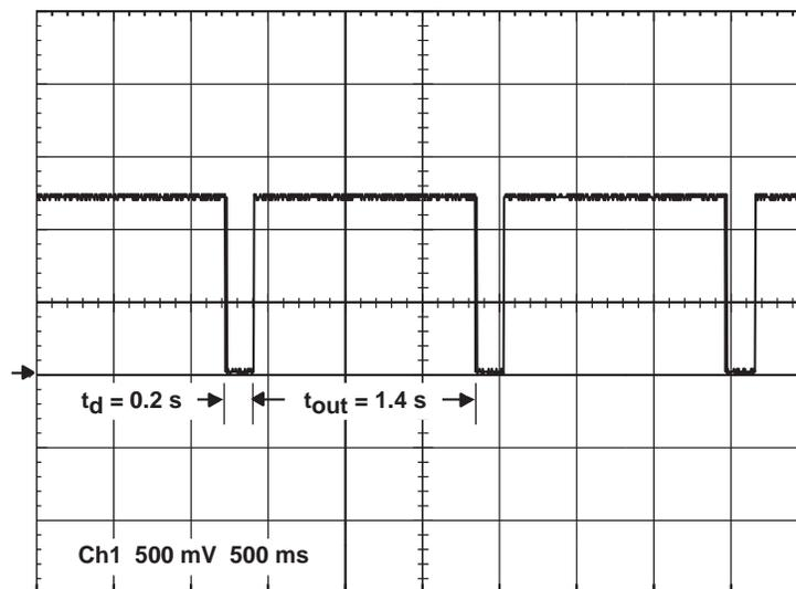
Figure 15. Signal Form at the  $\overline{\text{RESET}}$  Output
