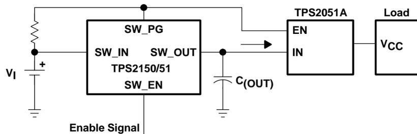
**Figure 10. Powering Large Load Through Power Sequencing for Loads Without an Enable**
