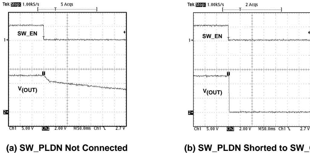
**Figure 11. Turnoff Output Voltage Waveforms With  $C_O = 4.7 \mu\text{F}$**
