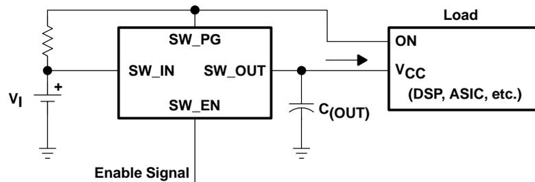
**Figure 8. Power Large Load Through Power Sequencing**
