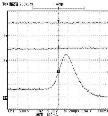
**Figure 4. Power Switch Power-Up Into a Pure Capacitive Load
