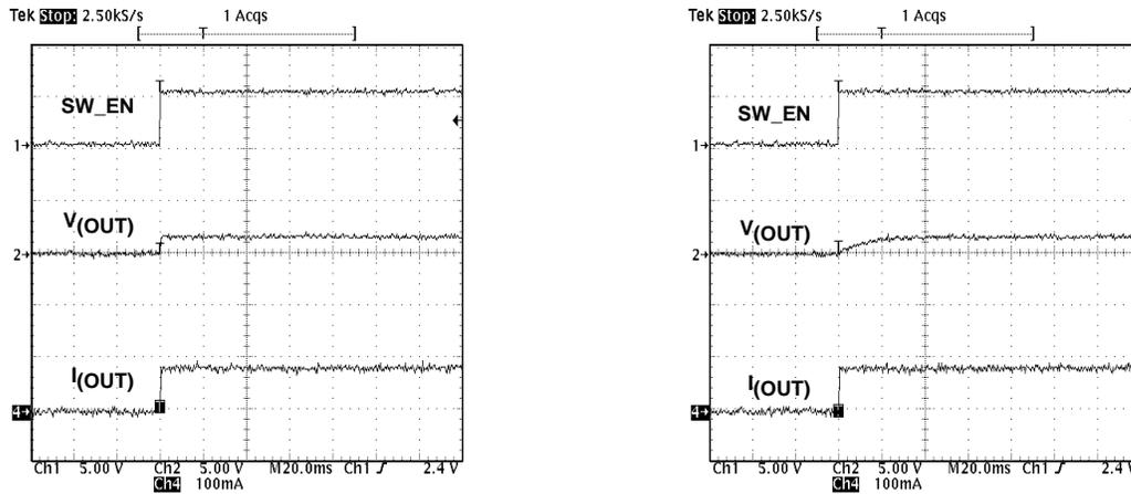
(a)  $C_O = 4.7 \mu\text{F}$ (b)  $C_O = 470 \mu\text{F}$ **Figure 7. Power Switch Power-Up With 20- $\Omega$  DC Load**
