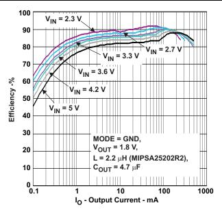
Figure 5. Efficiency vs Output Current (TPS62231)
