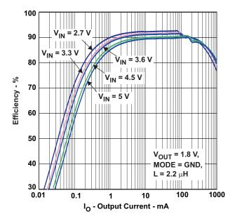
Figure 3. Efficiency vs Output Current (TPS62290)
