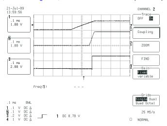
Figure 2. Shows Sequencing in Start up Waveform
