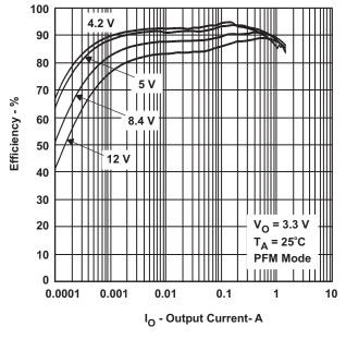
Figure 4. Efficiency vs Output Current (TPS62111)
