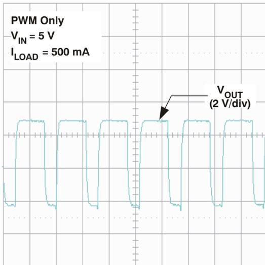
Figure 8. Switching Node Waveform
