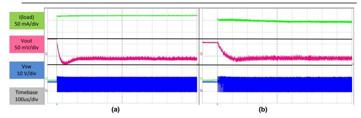
Figure 1. TPS62125 Load transient response using a (a) 10-μF and (b) 200-μF output capacitor
