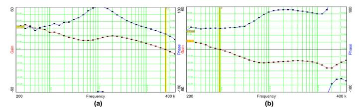
Figure 2. TPS62125 Closed-loop frequency response using a (a) 10-µF and (b) 200-µF output capacitor
