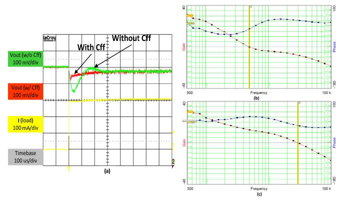
Figure 5. (a) Load Transient Response and (b) Closed-Loop Frequency Response without  $C_{\rm ff}$  and (c) with  $C_{\rm ff}$  = 120pF
