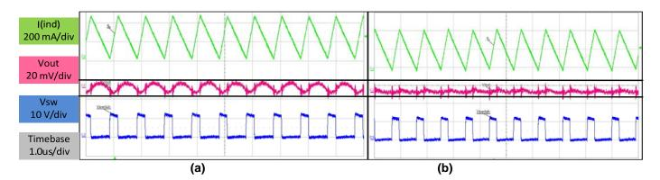
Figure 3. TPS62125 output voltage ripple using a (a) 10-µF and (b) 200-µF output capacitor
