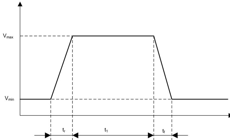
**Figure 2. Supply Profile 1 Timing Chart**
