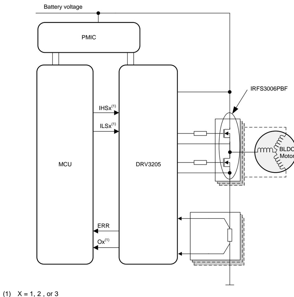
**Figure 1. Test Schematic**
