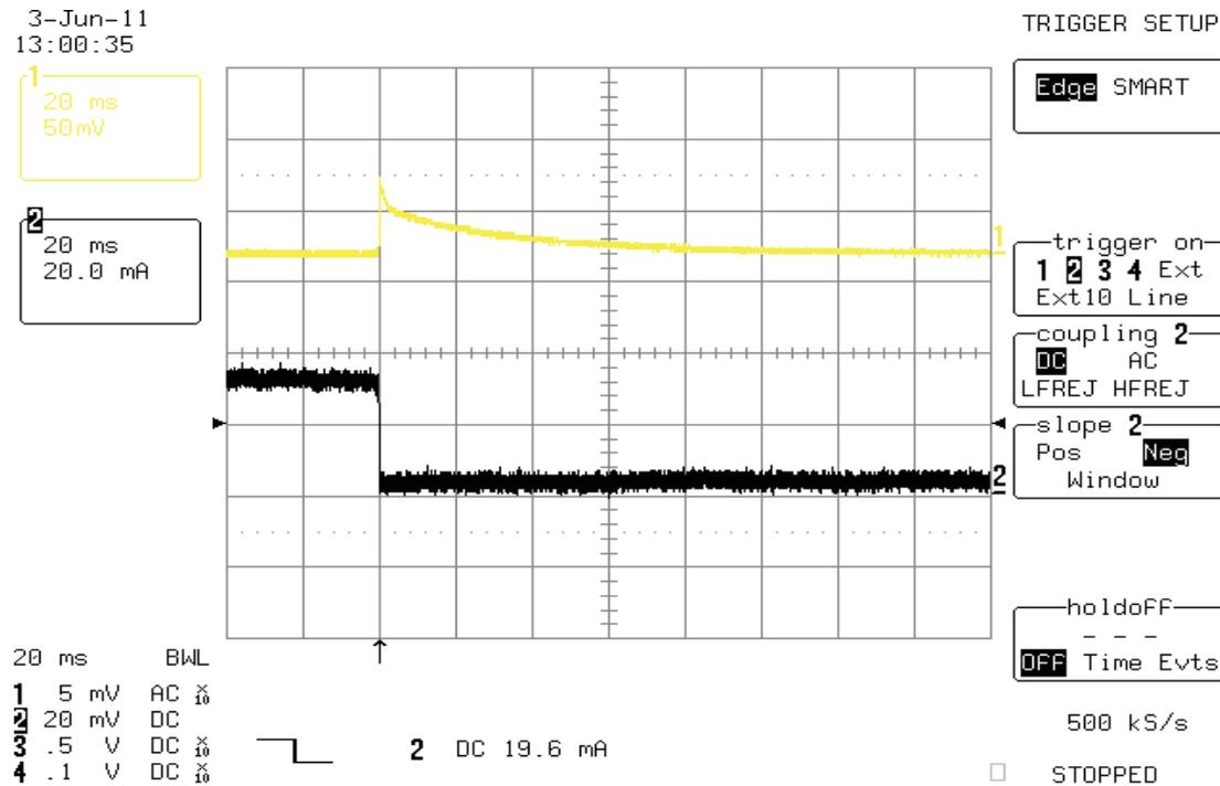
Figure 12. Load Transient, LDO : Vbat = 3.6 V with 30 mA to 0 mA Transient.
