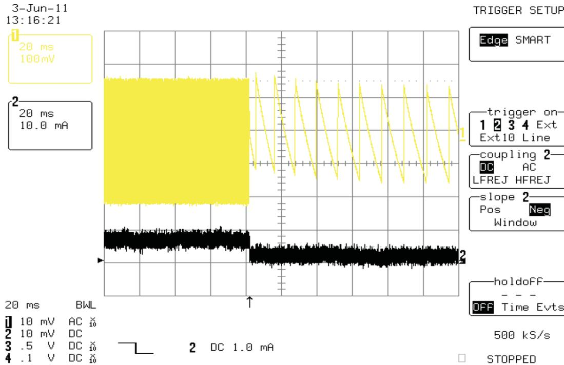
Figure 10. Load Transient, Boost : Vbat = 3.6 V with 5 mA to 0mA Transient, Constant 15 mA Load on LDO. CH3 Bstout CH4 I<sub>BOOST</sub>
