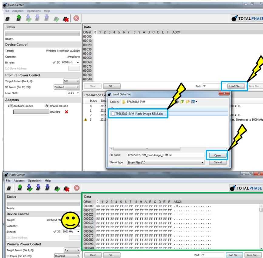
Figure 20. Loading Data Section of Flash Center
