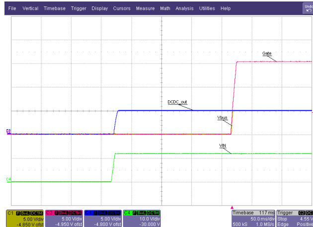
Figure 21. Raise V_{IN} With UFP Already Plugged In
