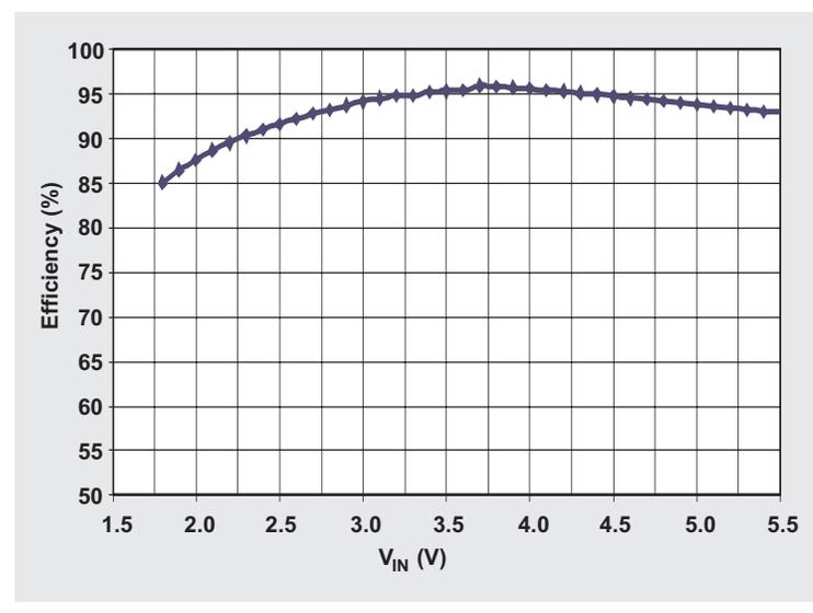
buck and boost functions into a single 3 × 3-mm QFN package, including switching FETs, compensation, and protection features. Only three external parts are required for operation: input and output capacitors and an inductor. The converter operates with a peak efficiency of 96% (see Figure 1). With a peak output current of 800 mA, it delivers
