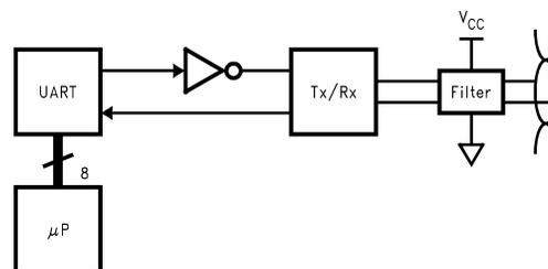
Figure 6. Typical SAE J1708 System Block Diagram
