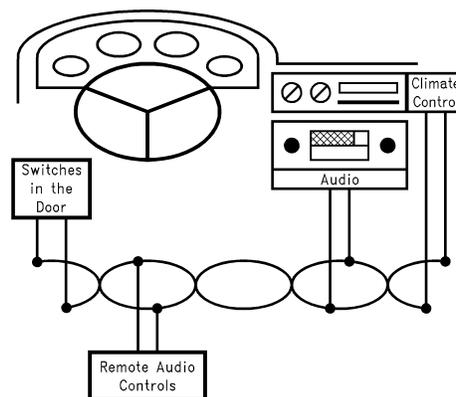
**Figure 1. Automobile Controls on a SAE J1708 Bus**
