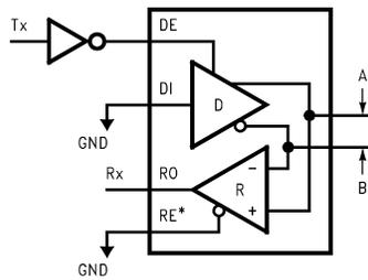
Figure 4. The DS75176B in a SAE J1708 Application
