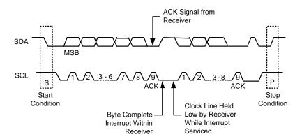
Figure 1. SMBus Transaction Format
