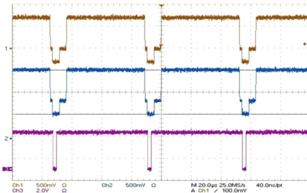
Ch1: 480i input at “Video In” BNC cable port (before  $R_s = 100 \Omega$ )
