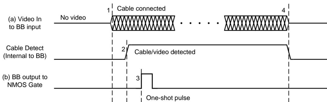
Figure 5. Example Timing Diagram to Pulse NMOS Switch to Pull-up VIN (Countermeasure Method #2)
