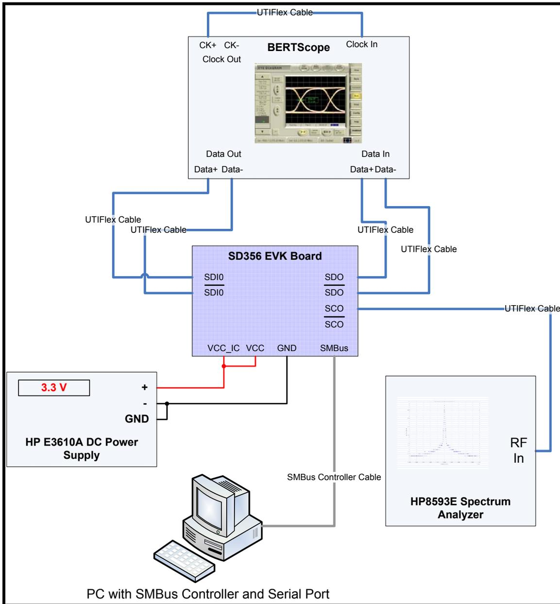
**Figure 2. Test setup for the SD356EVK board.**
