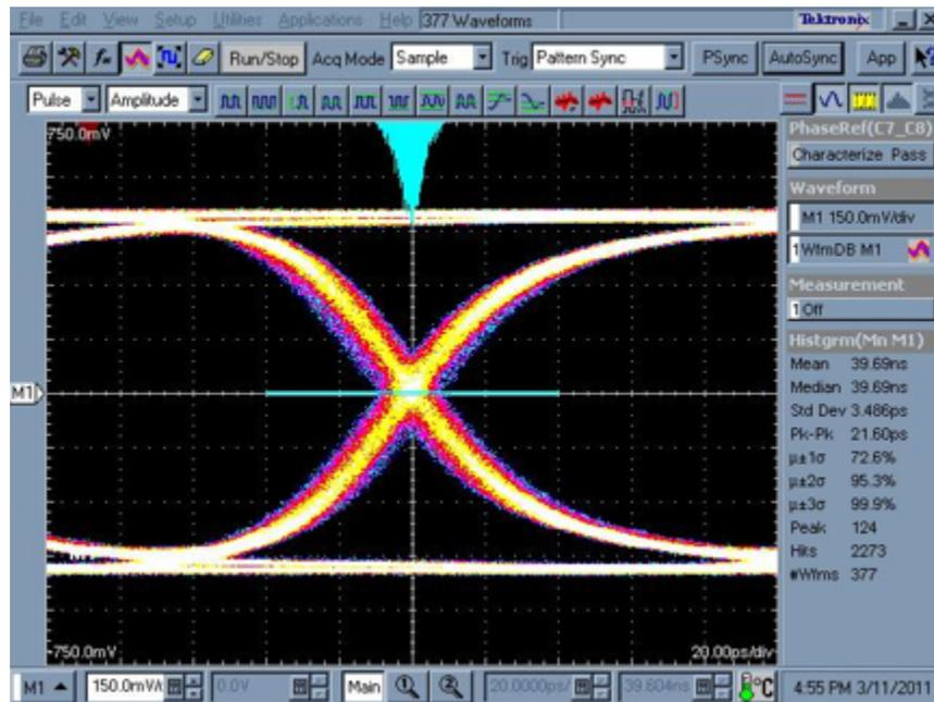
Figure 3. 6 Gbps Eye Diagram at SCOPE in SETUP
