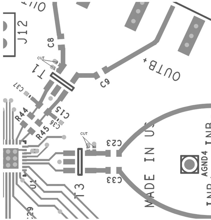
Figure 7. Trace Cuts for Differential Input and Output
