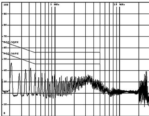
Figure 11. INE – CISPR/FCC Class B Average Scan
