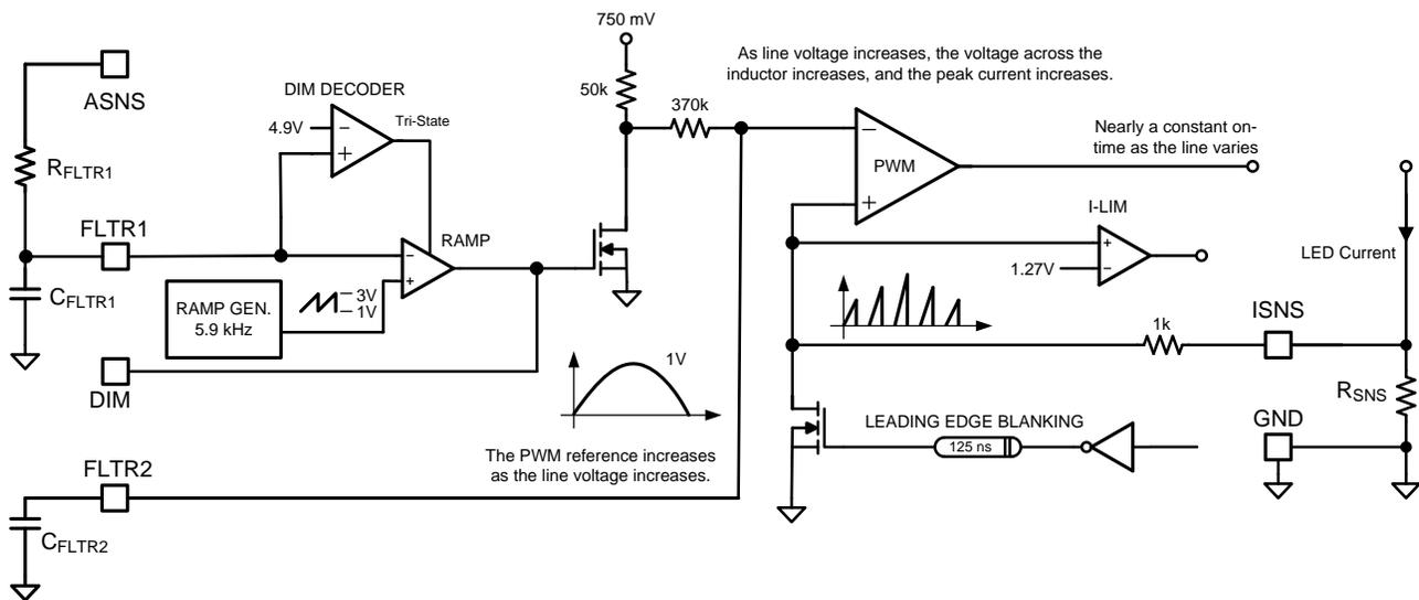
Figure 26. Typical Operation of FLTR2 Pin
