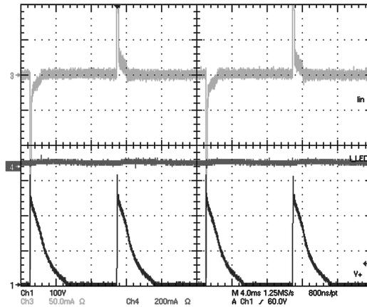
Figure 16. Forward phase circuit at 135° firing angle
