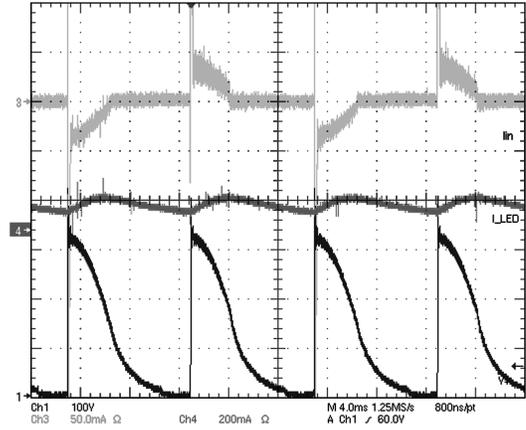
Figure 15. Forward phase circuit at 90° firing angle
