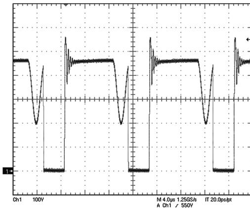
Figure 7. SW FET Drain Voltage Waveform
