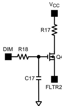
Figure 33. TRIAC Holding Circuit
