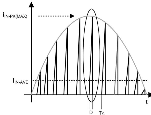
**Figure 27. DCM Flyback Current Waveforms**
