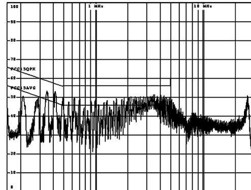
Figure 10. NEUTRAL – CISPR/FCC Class B Peak Scan
