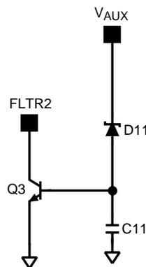
Figure 34. OVP Circuit
