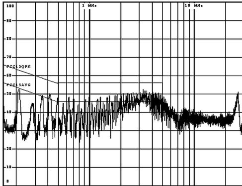
Figure 9. LINE – CISPR/FCC Class B Peak Scan
